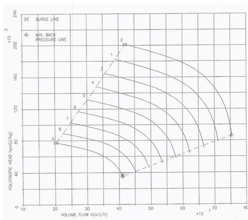
Figure 4.1 – MAN RB28–7 Performance curves
