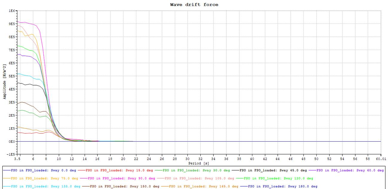
Figure 95 Sway wave drift force for FSO.
