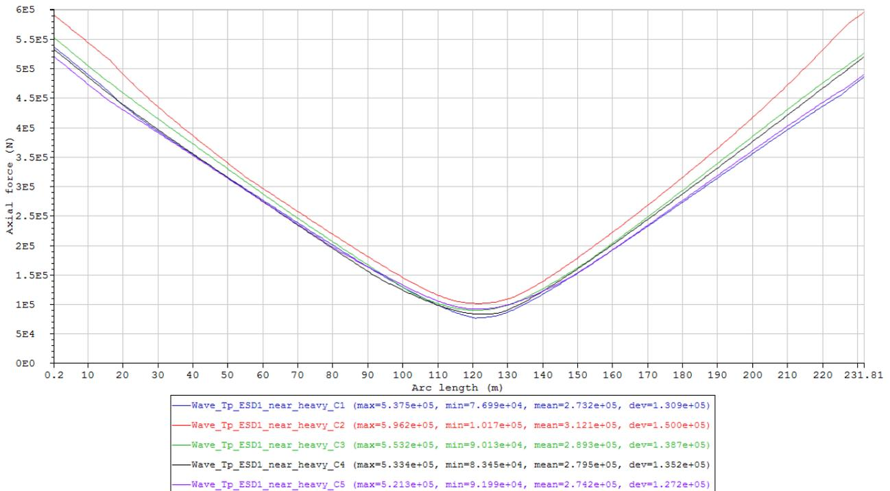
Figure 50 Maximum axial force envelope curves of the cases in Condition set – Wave\_Tp\_ESD1\_near\_heavy (Table 17).
