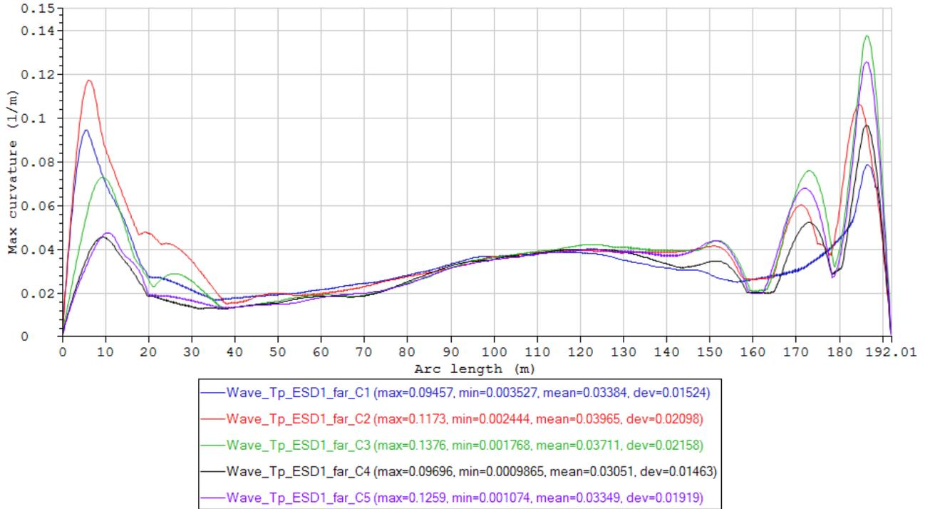
Figure 37 Maximum curvature envelope curves of the cases in Condition set – Wave\_Tp\_ESD1\_far (Table 15).
