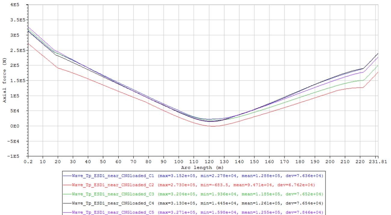
Figure 90 Minimum axial force envelope curves of the cases in Condition set – Wave\_Tp\_ESD1\_near\_CNGloaded (Table 23).
