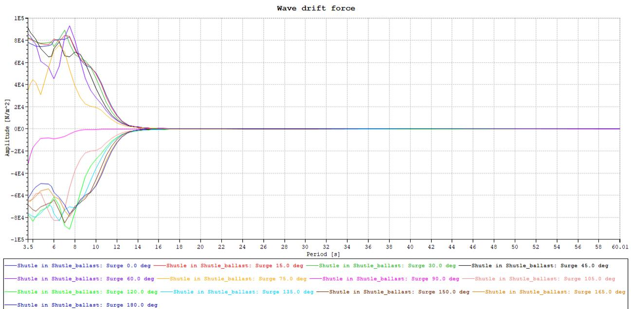
Figure 97 Surge wave drift force for GASVESSEL.
