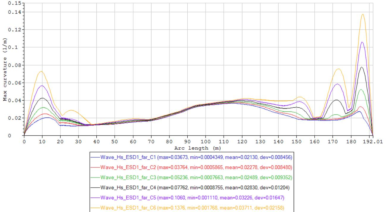
Figure 31 Maximum curvature envelope curves of the cases in Condition set – Wave\_Hs\_ESD1\_far (Table 15).
