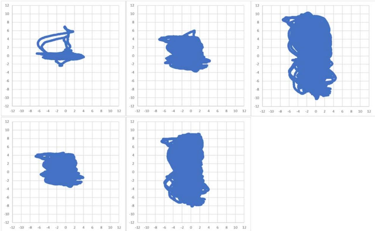
Figure 17 Surge (vertical) and sway (horizontal) motion relative to mean FSO turret position, for all  $T_p$  for the five environment cases in Table 29.
