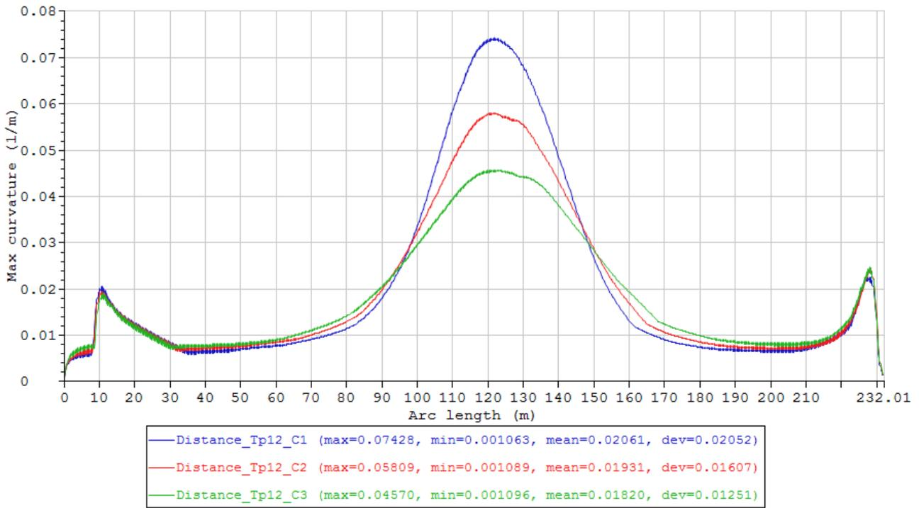
Figure 79 Maximum curvature envelope curves of the cases in Condition set – Distance\_Tp12 (Table 23).
