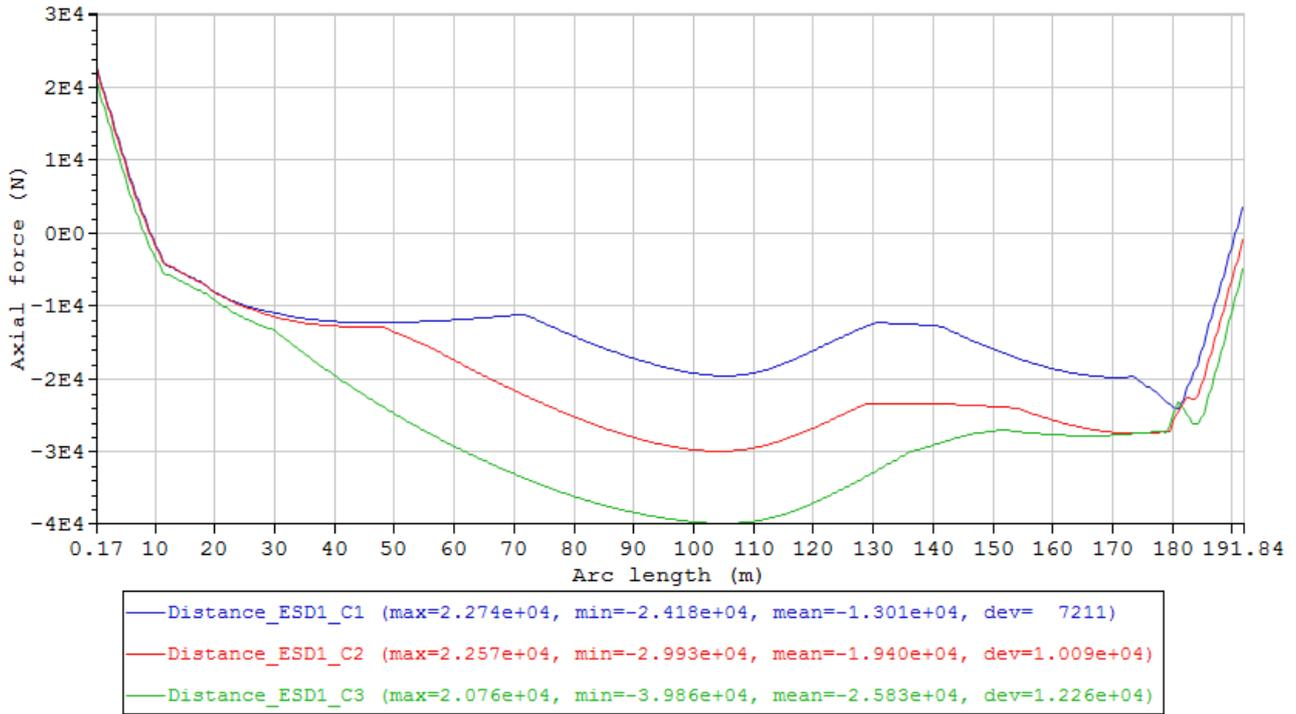
Figure 27 Minimum axial force envelope curves of the cases in Condition set - Distance\_ESD1 (Table 15).
