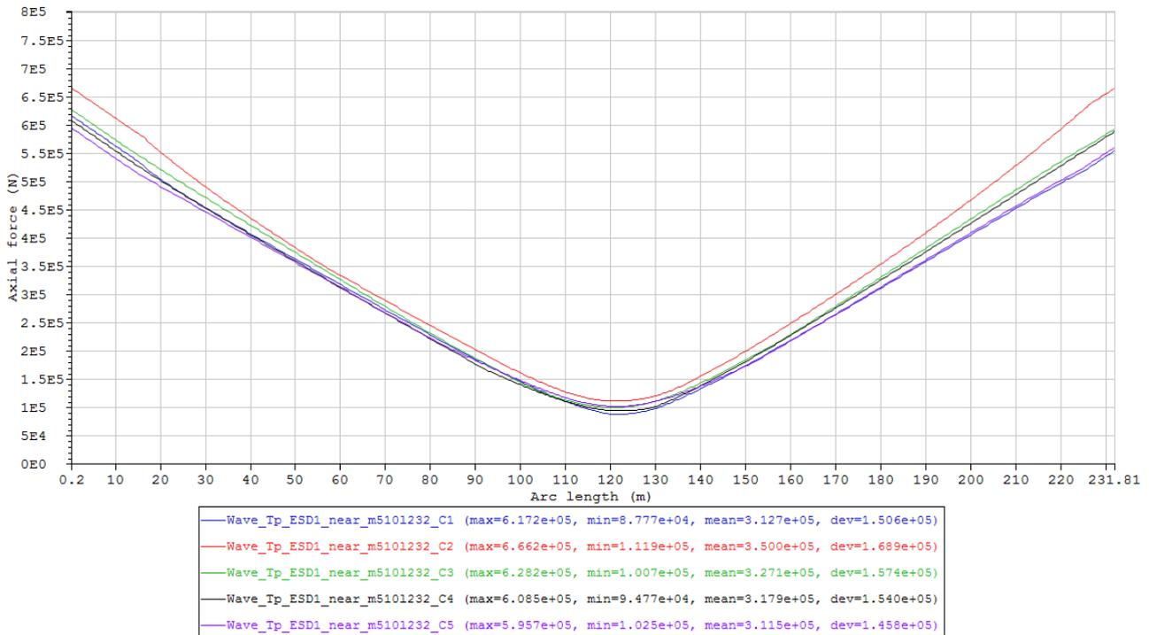
Figure 74 Maximum axial force envelope curves of the cases in Condition set – Wave\_Tp\_ESD1\_near\_m5101232 (Table 21).
