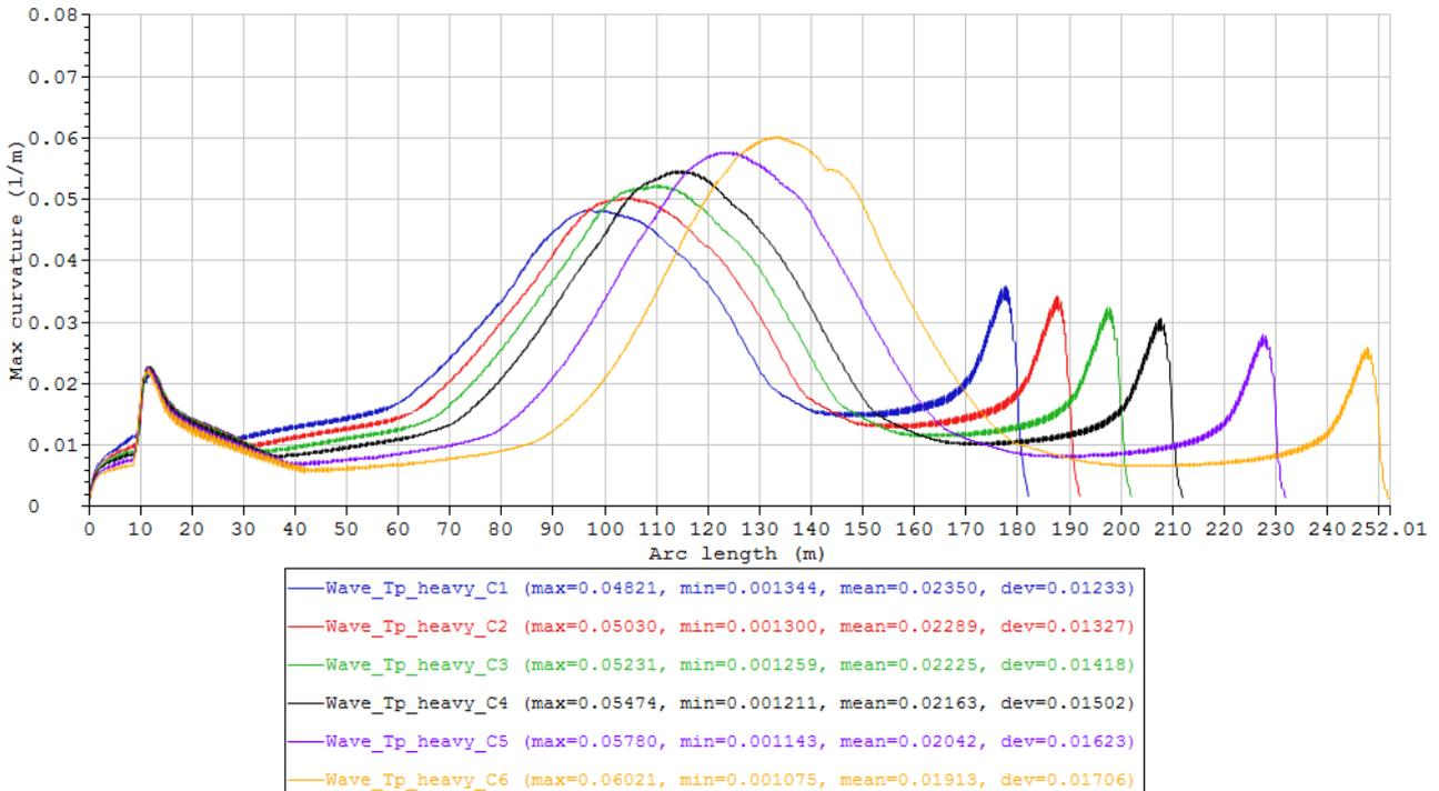
Figure 40 Maximum curvature envelope curves of the cases in Condition set – Wave\_Tp\_heavy (Table 17).
