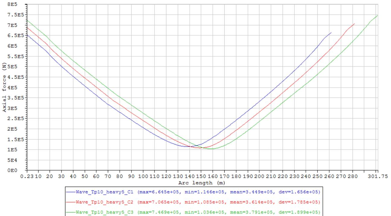
Figure 56 Maximum axial force envelope curves of the cases in Condition set - Wave\_Tp10\_heavy5, first 3 cases with length variation (Table 19).
