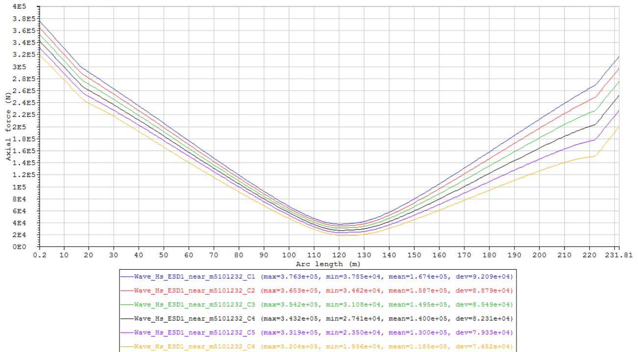
Figure 69 Minimum axial force envelope curves of the cases in Condition set – Wave\_Hs\_ESD1\_near\_m5101232 (Table 21).
