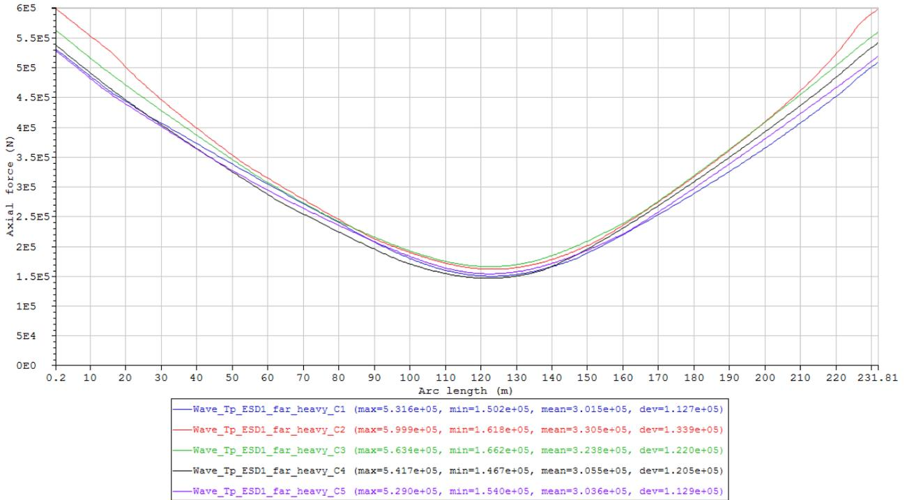
Figure 53 Maximum axial force envelope curves of the cases in Condition set – Wave\_Tp\_ESD1\_far\_heavy (Table 17).
