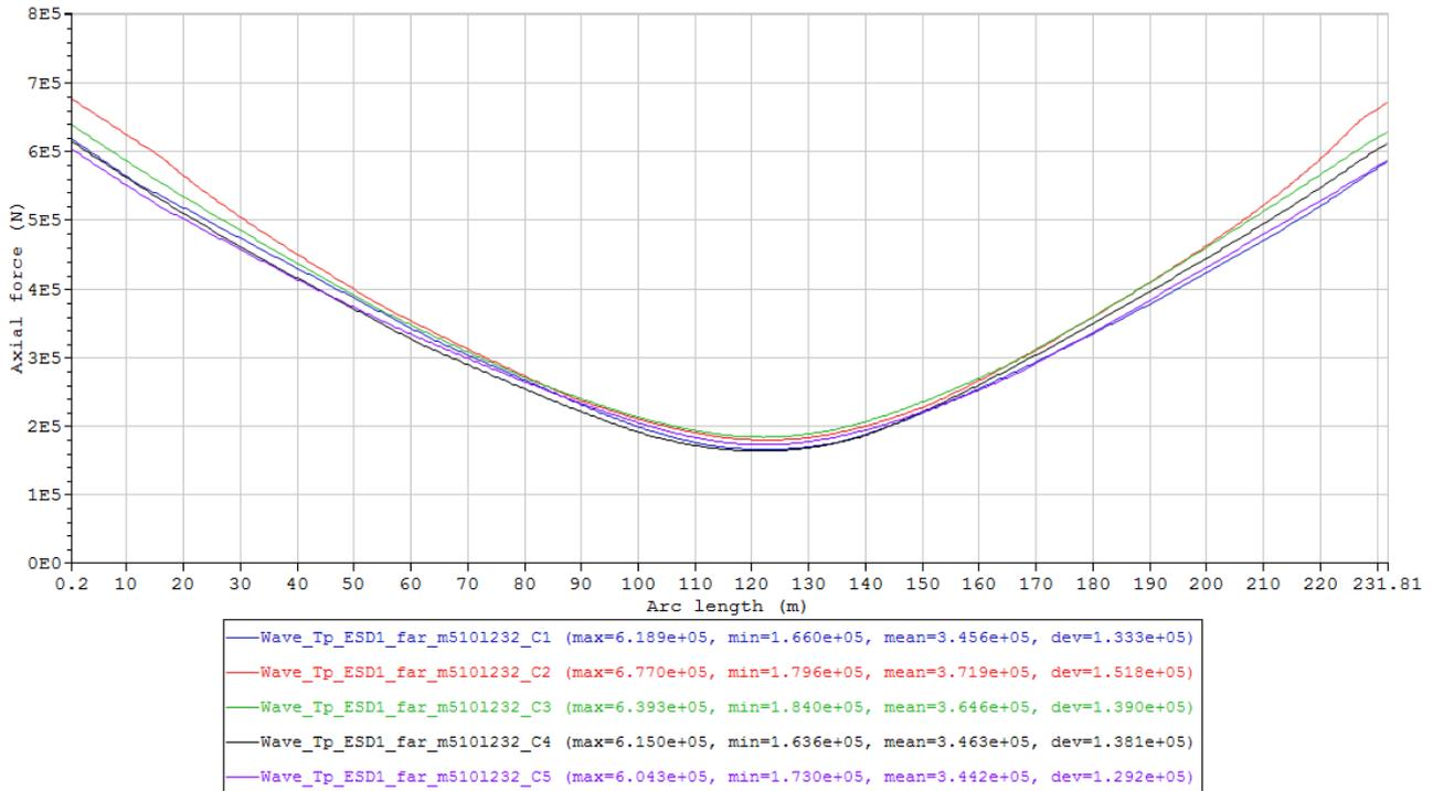
Figure 77 Maximum axial force envelope curves of the cases in Condition set – Wave\_Tp\_ESD1\_far\_m5101232 (Table 21).
