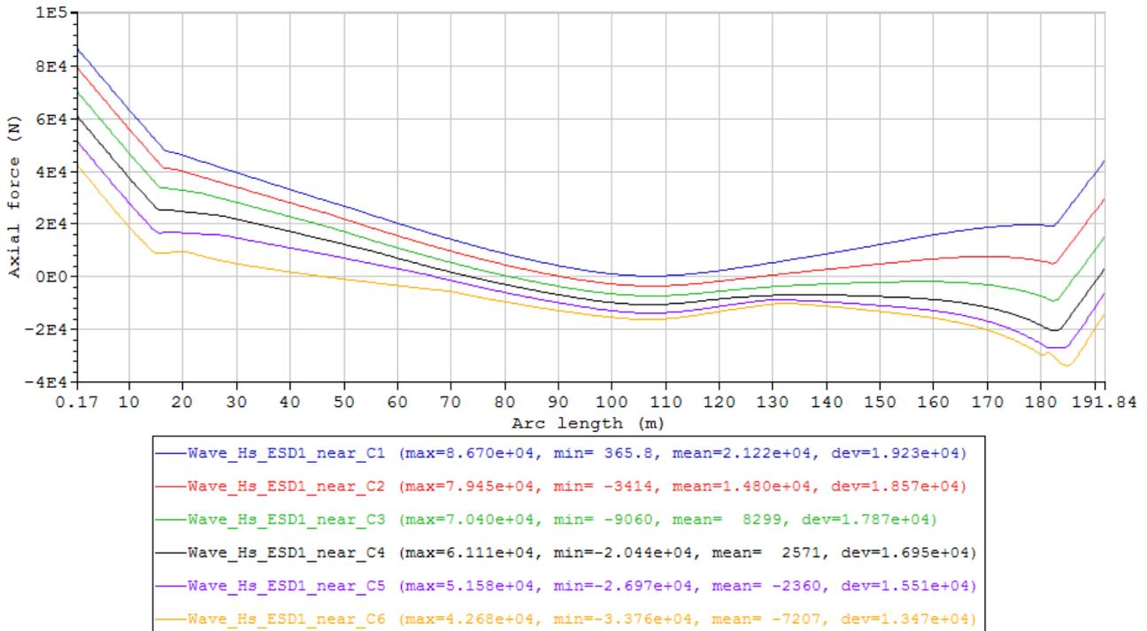
Figure 30 Minimum axial force envelope curves of the cases in Condition set – Wave\_Hs\_ESD1\_near (Table 15).
