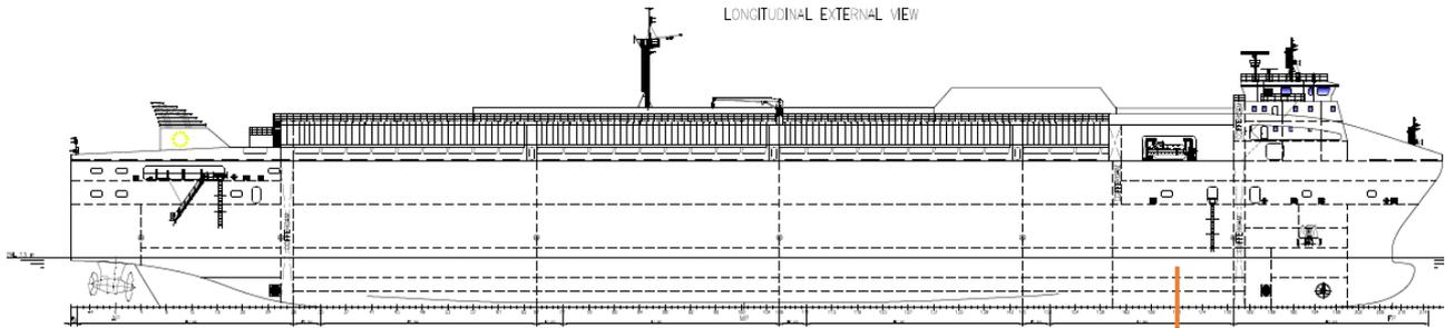
Figure 12 The GA showing the assumed location of the middle of the turret as a red line.
