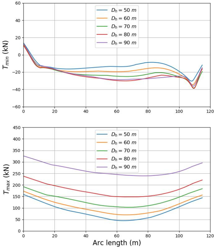
Fig. 14 Dynamic tension envelope curves (minimum and maximum) along the loading hose arc length,  $D_h$  varies from 50 m to 90 m.  $L_h = 115$  m. FSO at the left side, CNG vessel at the right side.
