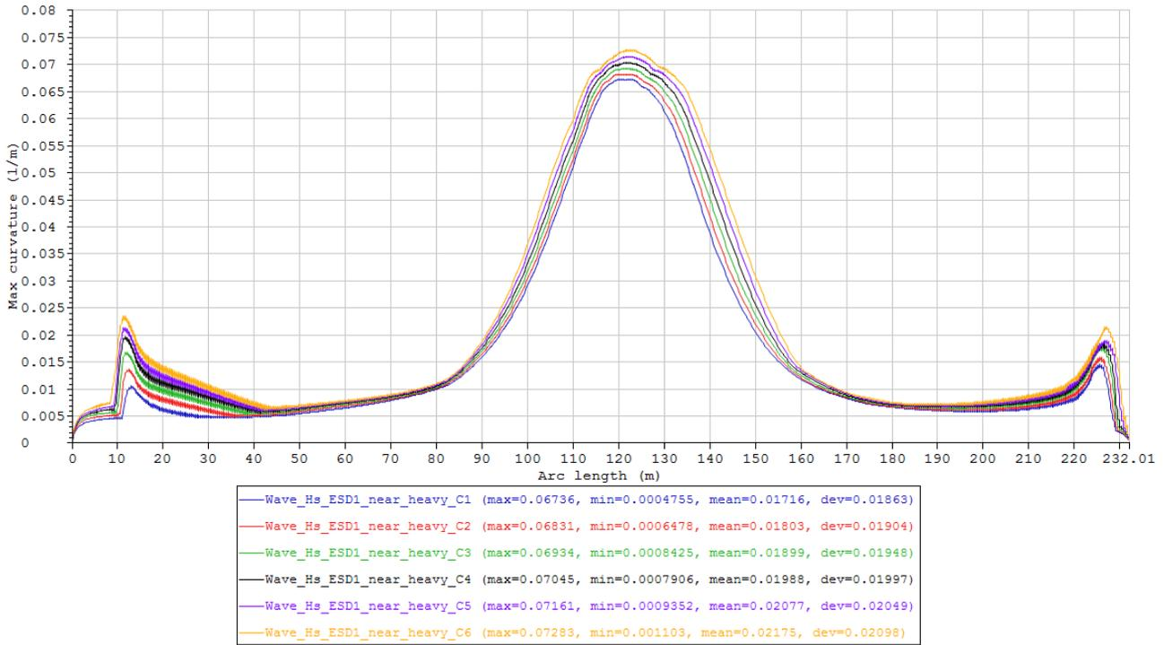
Figure 43 Maximum curvature envelope curves of the cases in Condition set – Wave\_Hs\_ESD1\_near\_heavy (Table 17).
