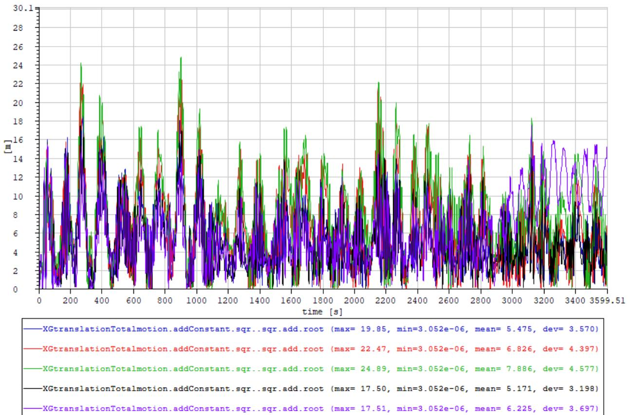
Figure 15 The turret offset for the 5 collinear 100 years environment cases.
