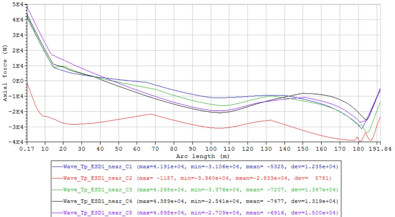
Figure 36 Minimum axial force envelope curves of the cases in Condition set – Wave\_Tp\_ESD1\_near (Table 15).
