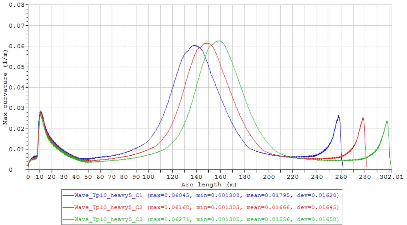
Figure 55 Maximum curvature envelope curves of the cases in Condition set – Wave\_Tp10\_heavy5, first 3 cases with length variation (Table 19).
