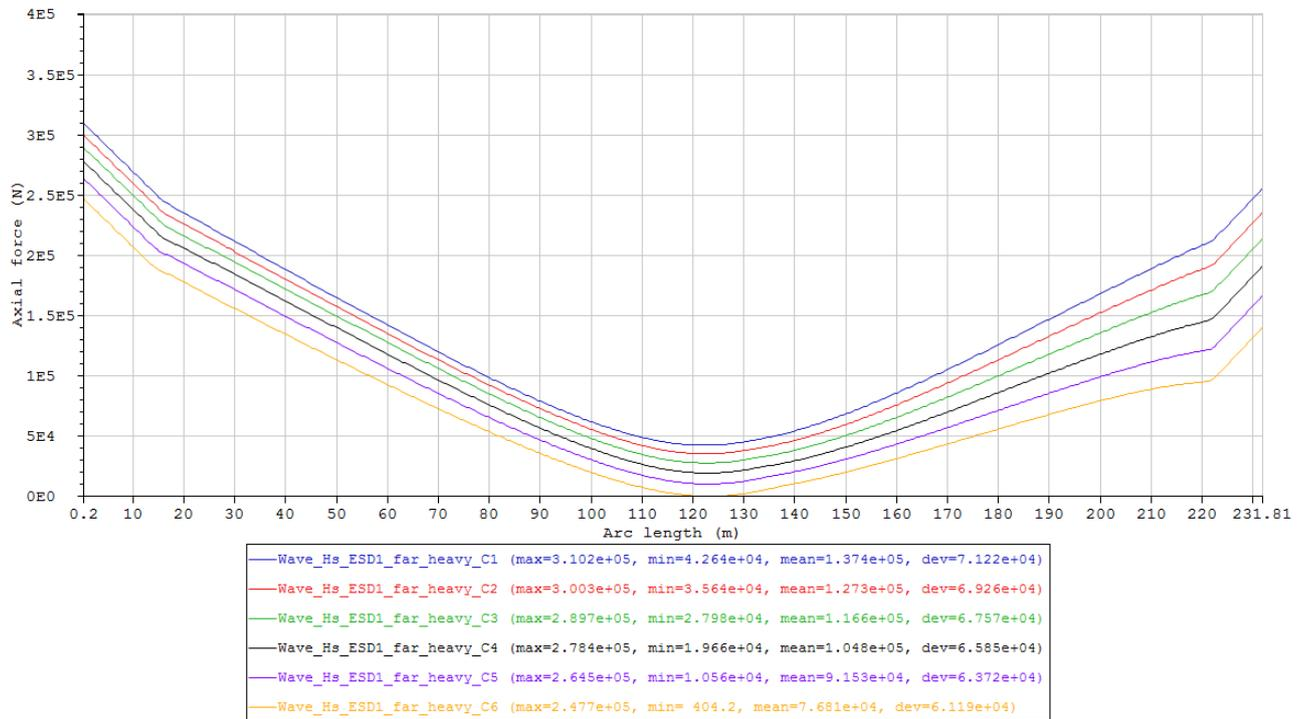
Figure 48 Minimum axial force envelope curves of the cases in Condition set – Wave\_Hs\_ESD1\_far\_heavy (Table 17).
