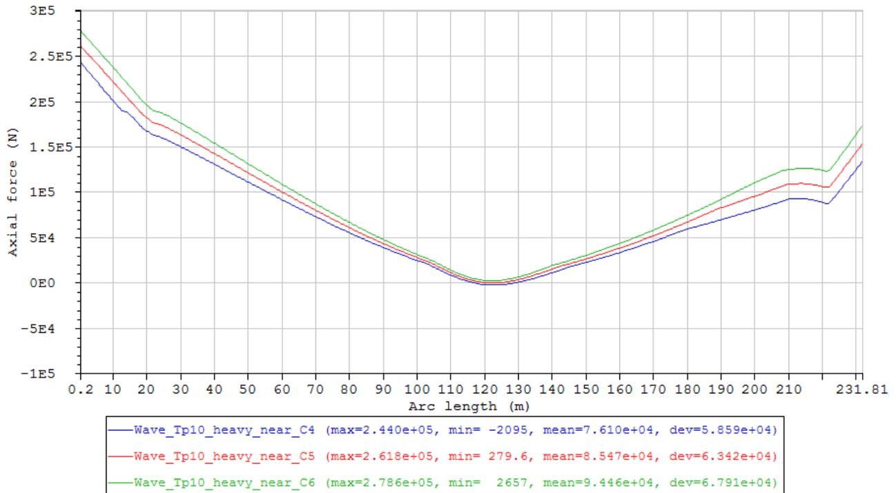
Figure 66 Minimum axial force envelope curves of the cases in Condition set – Wave\_Tp10\_heavy5\_near, last 3 cases with mass/length variation (Table 19).
