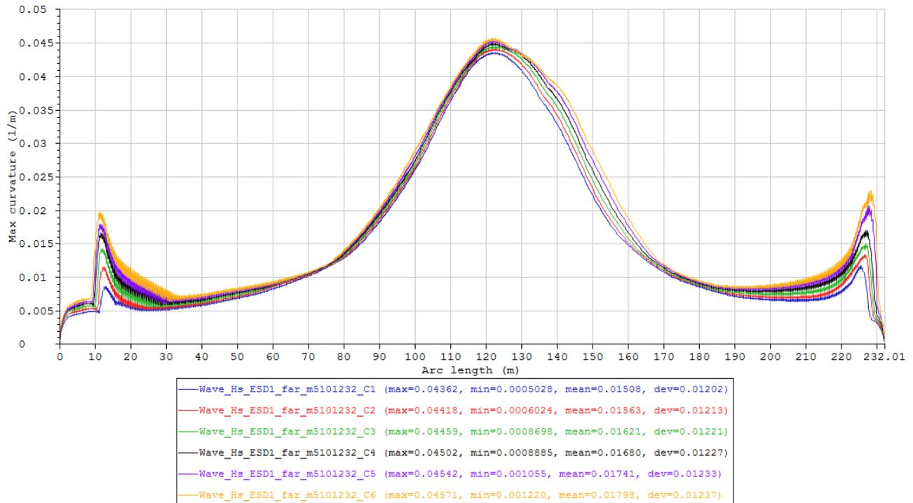
Figure 70 Maximum curvature envelope curves of the cases in Condition set – Wave\_Hs\_ESD1\_far\_m5101232 (Table 21).
