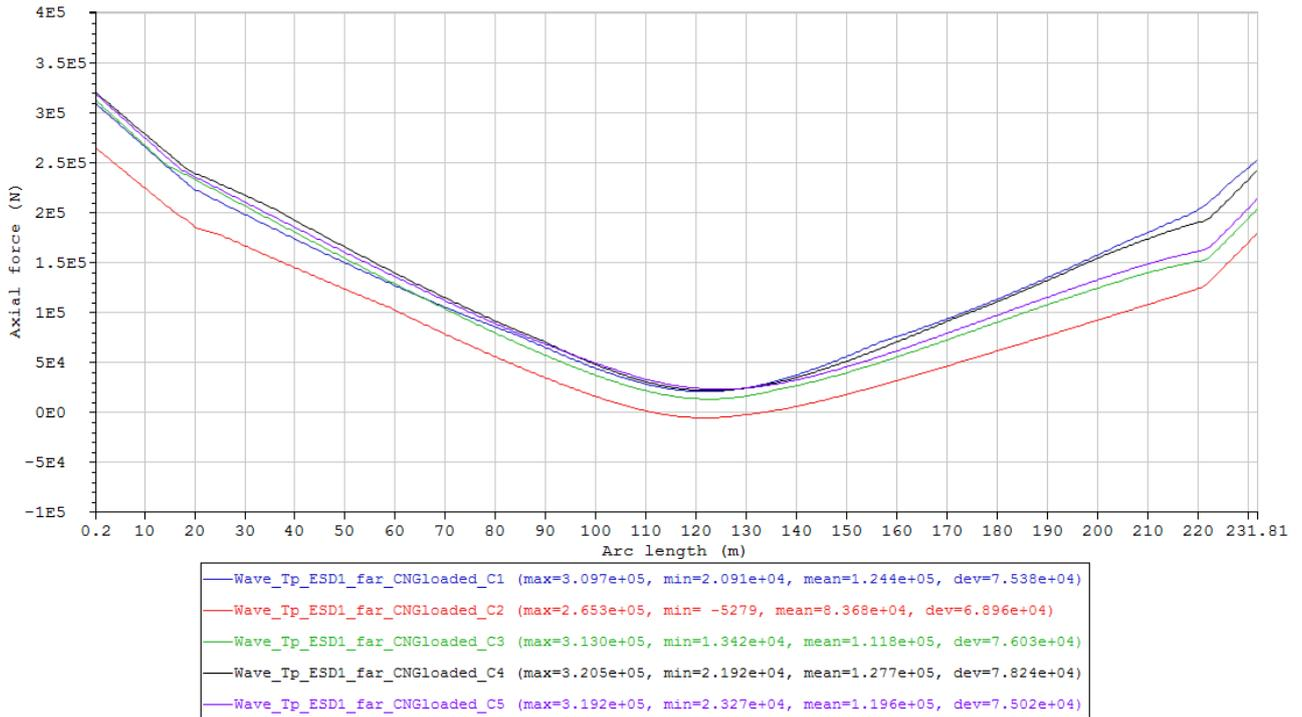
Figure 93 Minimum axial force envelope curves of the cases in Condition set – Wave\_Tp\_ESD1\_far\_CNGloaded (Table 23).
