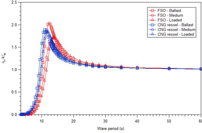
Fig. 9 Roll motion RAOs for the different hull variants and loading conditions in beam waves ( $\beta = 90$  deg). The roll RAO is given in rad/m.
