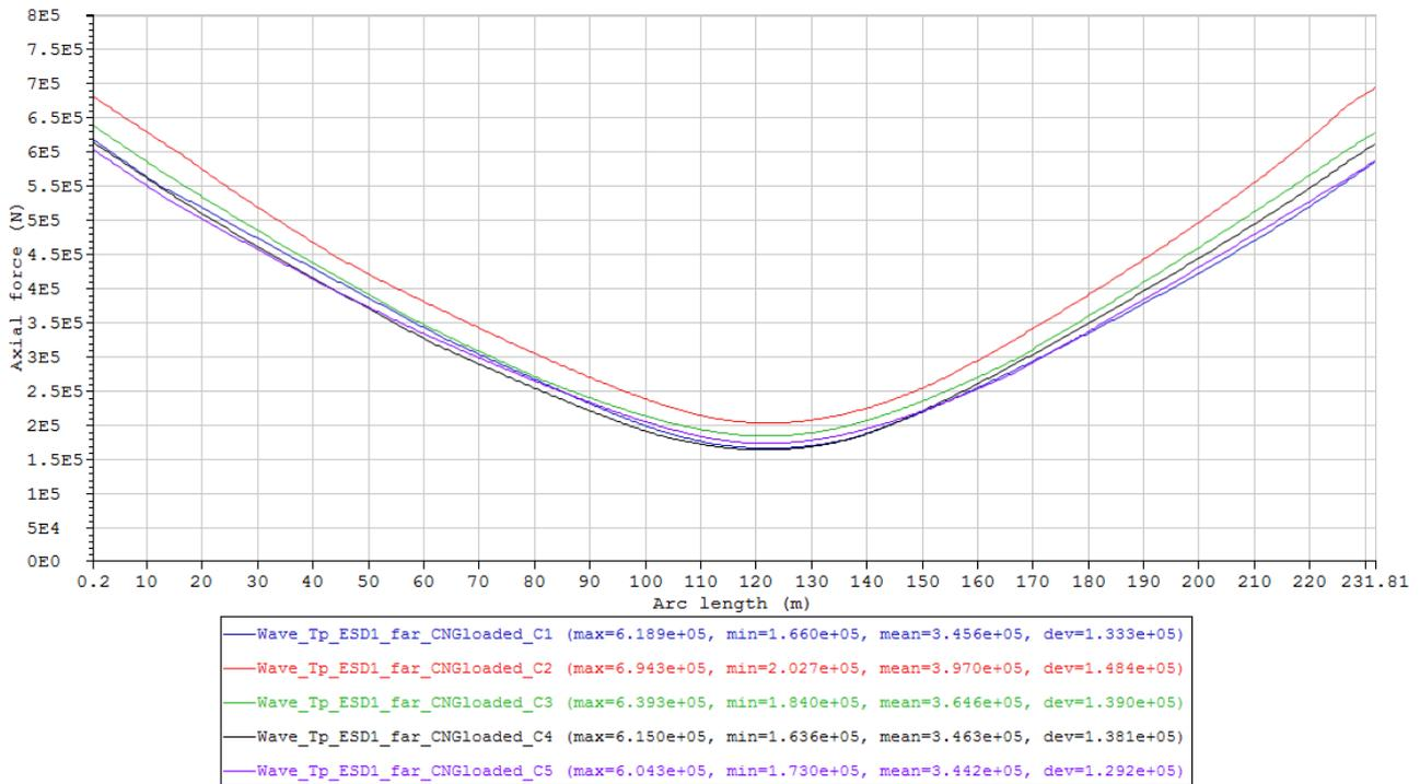
Figure 92 Maximum axial force envelope curves of the cases in Condition set – Wave\_Tp\_ESD1\_far\_CNGloaded (Table 23).
