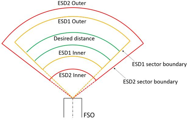
Fig. 4 Illustration of offloading sectors behind FSO.
