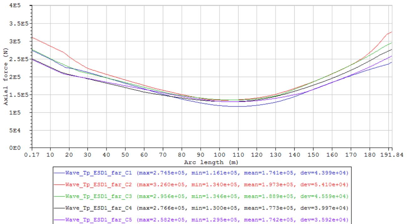
Figure 38 Maximum axial force envelope curves of the cases in Condition set – Wave\_Tp\_ESD1\_far (Table 15).
