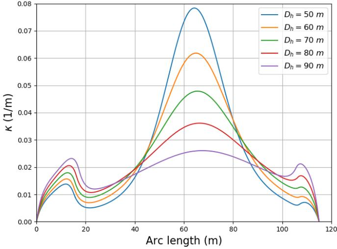
Fig. 11 Static curvature along the loading hose arc length,  $D_h$  varies from 50 m to 90 m.  $L_h = 115$  m. FSO at the left side, CNG vessel at the right side.
