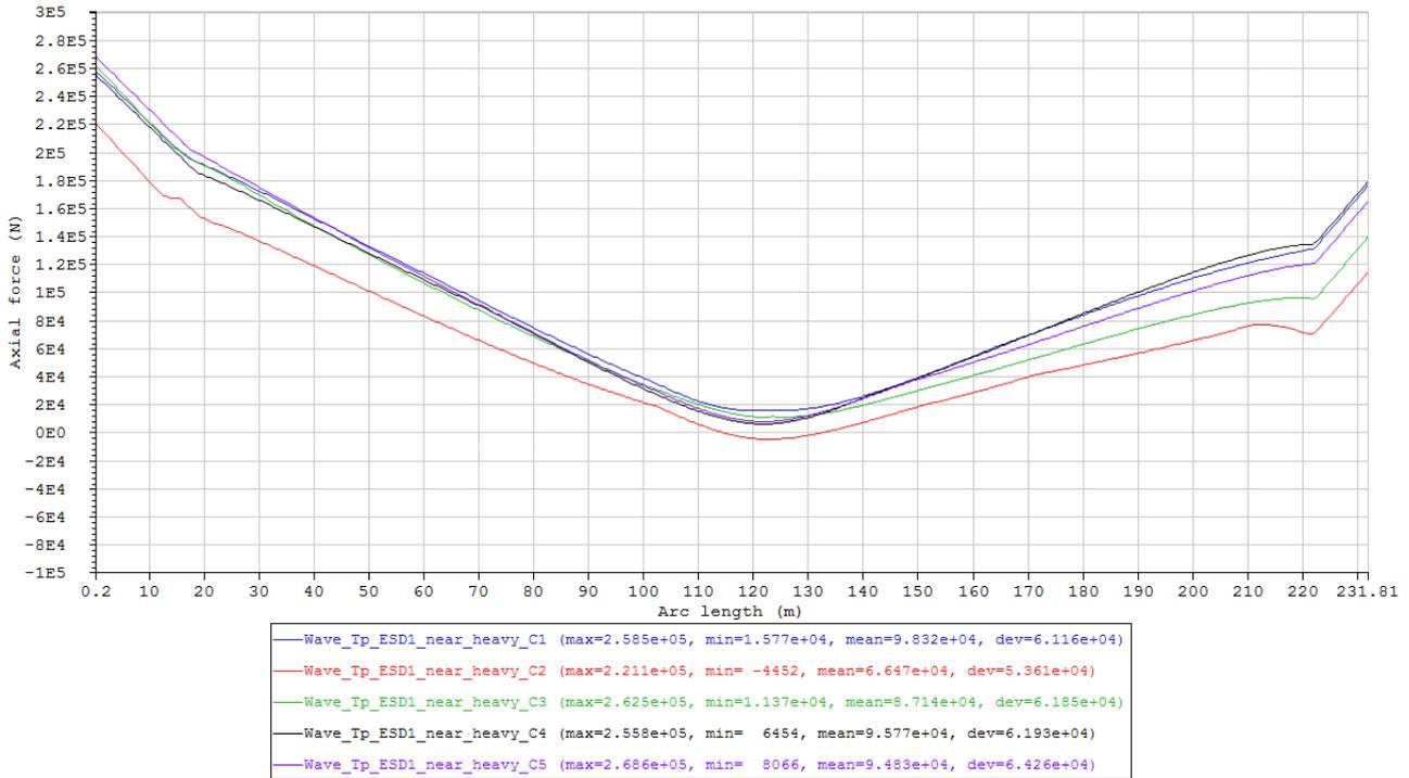
Figure 51 Minimum axial force envelope curves of the cases in Condition set – Wave\_Tp\_ESD1\_near\_heavy (Table 17).
