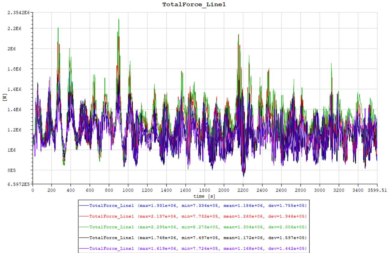
Figure 16 Line tension in the most exposed line for the 5 collinear 100 years environment cases.
