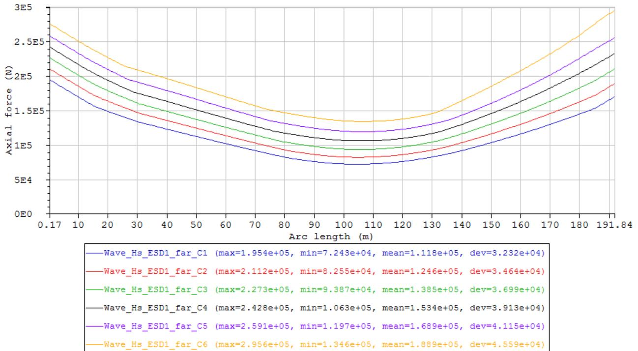
Figure 32 Maximum axial force envelope curves of the cases in Condition set – Wave\_Hs\_ESD1\_far (Table 15).
