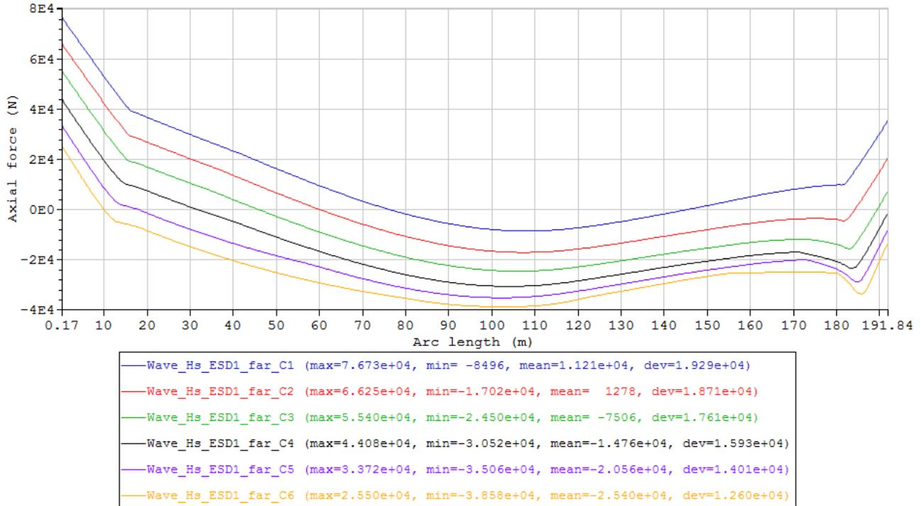
Figure 33 Minimum axial force envelope curves of the cases in Condition set – Wave\_Hs\_ESD1\_far (Table 15).
