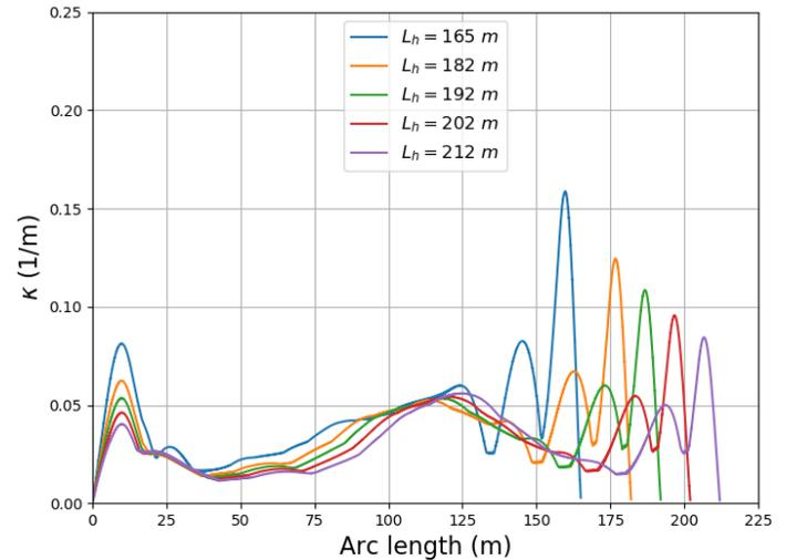
Fig. 16 Dynamic curvature envelope along the loading hose arc length,  $L_h$  varies from 165 m to 212 m.  $D_h = 100$  m. FSO at the left side, CNG vessel at the right side.
