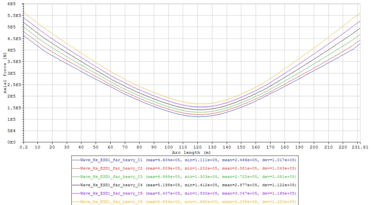
Figure 47 Maximum axial force envelope curves of the cases in Condition set – Wave\_Hs\_ESD1\_far\_heavy (Table 17).
