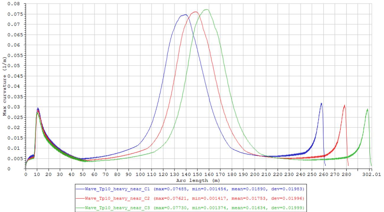
Figure 61 Maximum curvature envelope curves of the cases in Condition set – Wave\_Tp10\_heavy5\_near, first 3 cases with length variation (Table 19).
