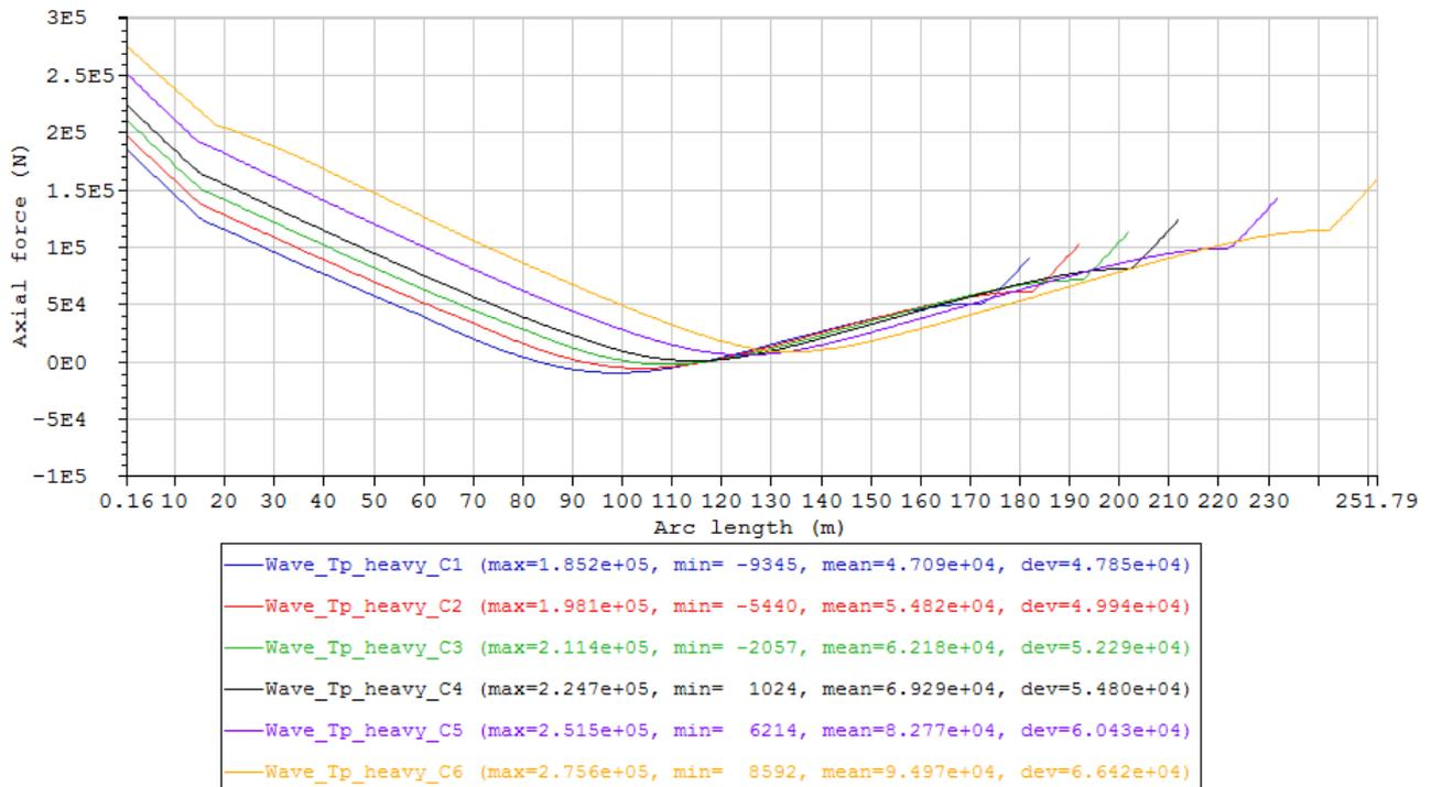
Figure 42 Minimum axial force envelope curves of the cases in Condition set – Wave\_Tp\_heavy (Table 17).
