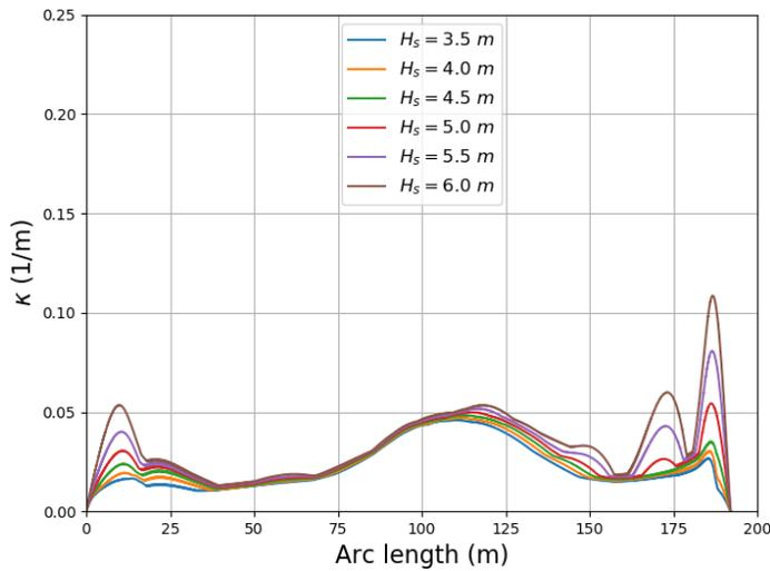
Fig. 18 Dynamic curvature envelope along the loading hose arc length.  $H_s$  varies from 3.5 m to 6.0 m,  $T_p = 13.6$  s.  $L_h = 192$  m,  $D_h = 100$  m. FSO at the left side, CNG vessel at the right side.
