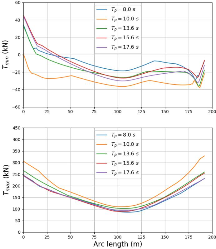
Fig. 21 Dynamic tension envelope curves (minimum and maximum) along the loading hose arc length.  $T_p$  varies from 8.0 s to 17.6 s,  $H_s = 6$  m.  $L_h = 192$  m,  $D_h = 100$  m. FSO at the left side, CNG vessel at the right side.
