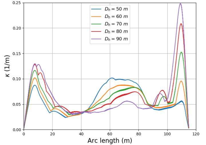
Fig. 13 Dynamic curvature envelope along the loading hose arc length,  $D_h$  varies from 50 m to 90 m.  $L_h = 115$  m. FSO at the left side, CNG vessel at the right side.
