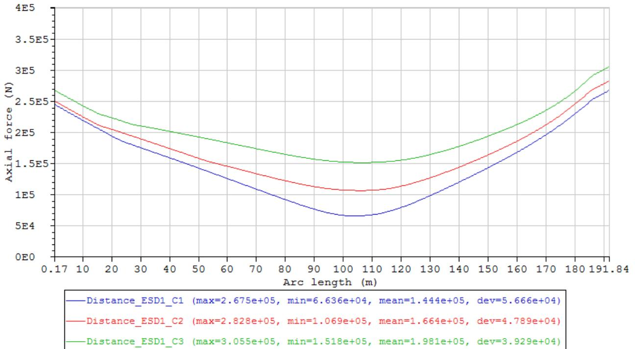
Figure 26 Maximum axial force envelope curves of the cases in Condition set - Distance\_ESD1 (Table 15).
