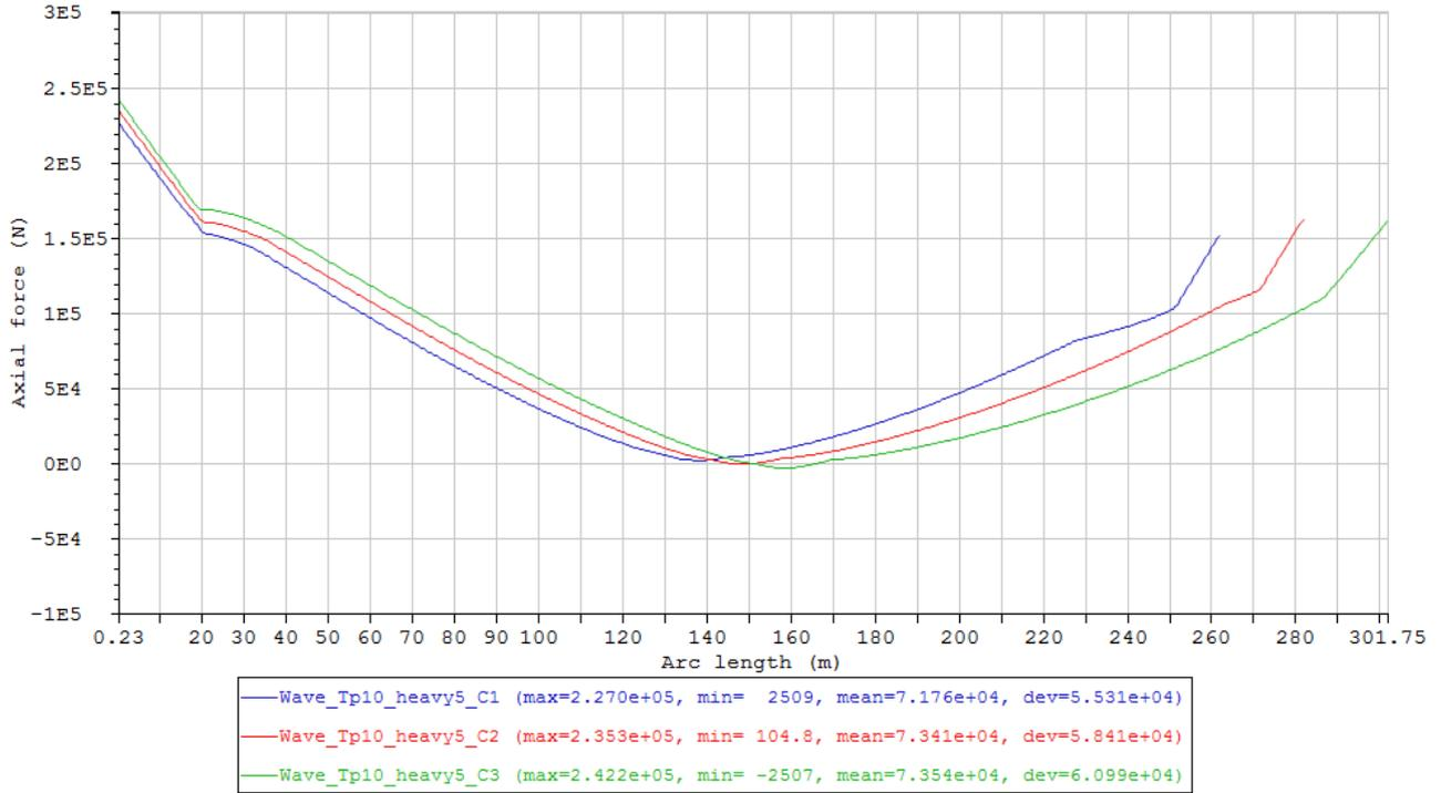
Figure 57 Minimum axial force envelope curves of the cases in Condition set - Wave\_Tp10\_heavy5, first 3 cases with length variation (Table 19).
