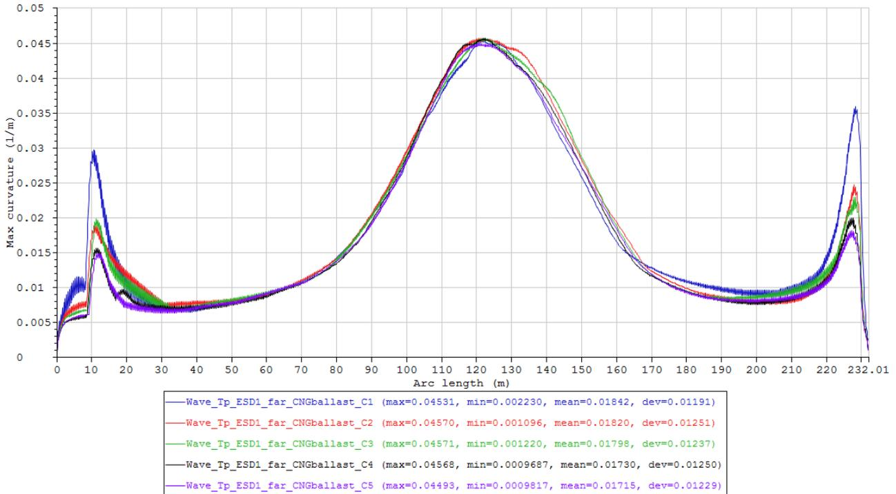
Figure 85 Maximum curvature envelope curves of the cases in Condition set – Wave\_Tp\_ESD1\_far\_CNGballast (Table 23).
