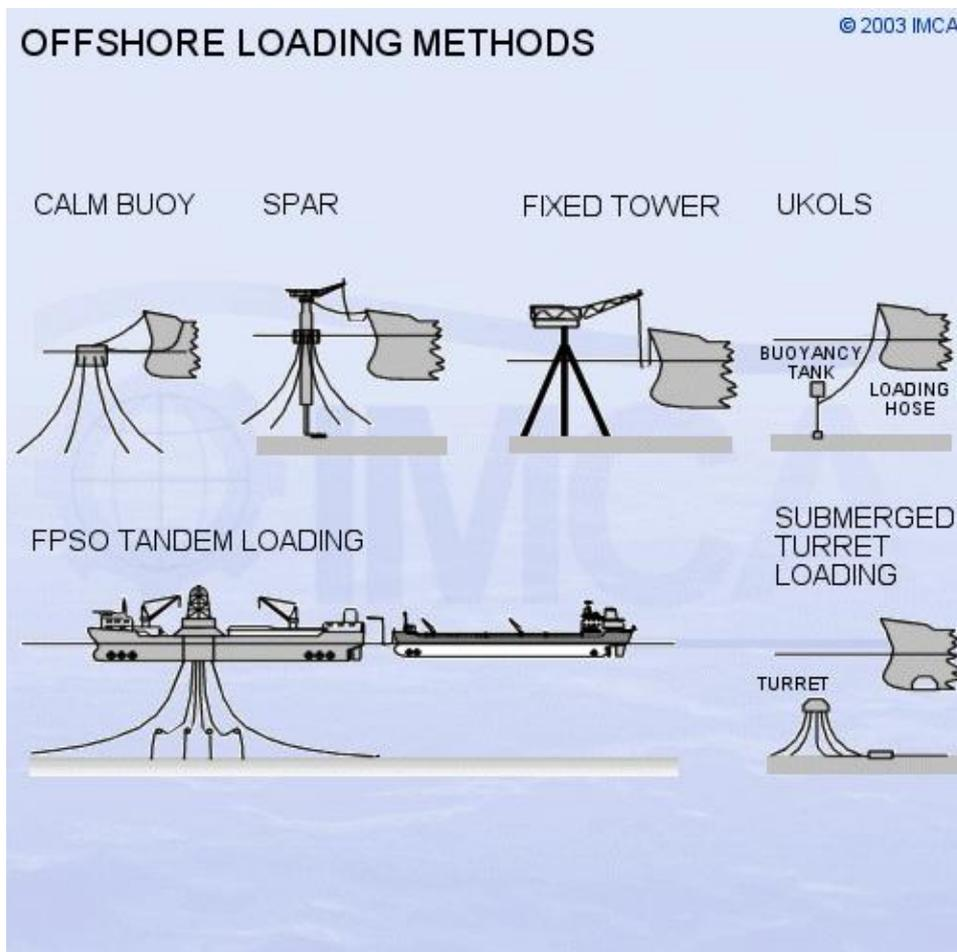
Figure 6 Sketch of different offshore loading methods. [4]
