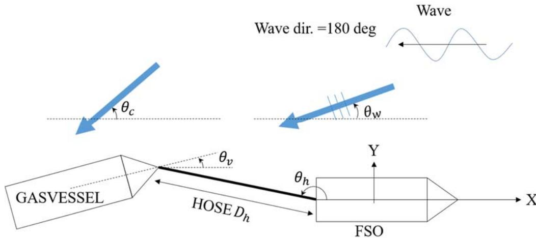
Figure 8 Coordinate system and operational parameters of a tandem loading/unloading system.
