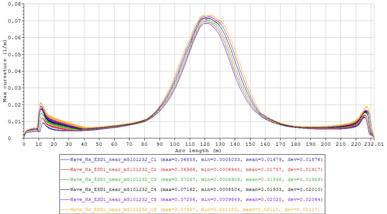
Figure 67 Maximum curvature envelope curves of the cases in Condition set – Wave\_Hs\_ESD1\_near\_m5101232 (Table 21).
