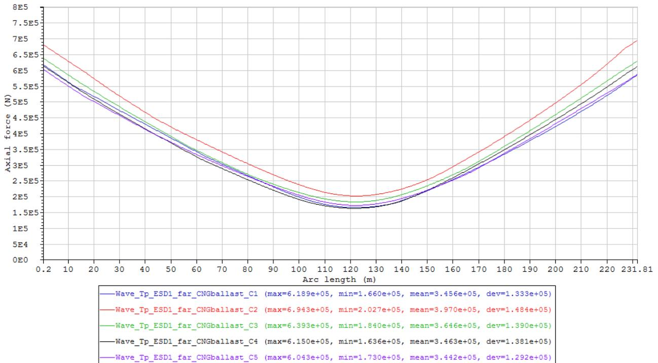
Figure 86 Maximum axial force envelope curves of the cases in Condition set – Wave\_Tp\_ESD1\_far\_CNGballast (Table 23).
