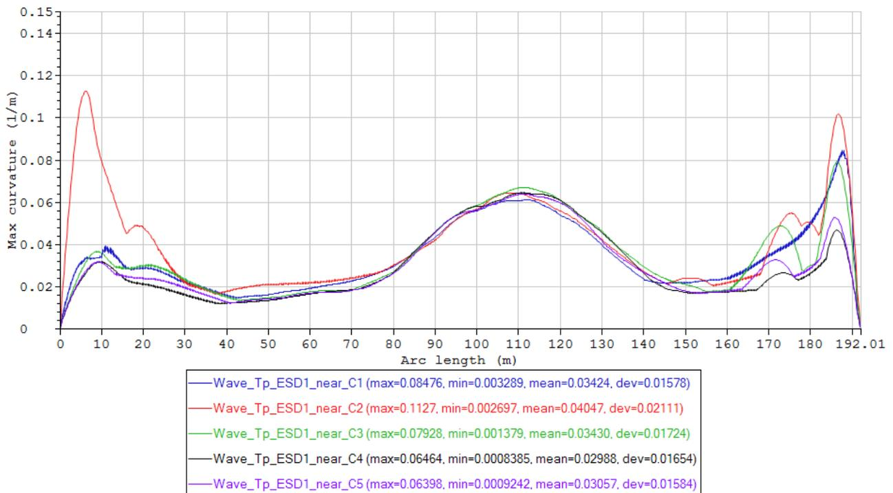
Figure 34 Maximum curvature envelope curves of the cases in Condition set – Wave\_Tp\_ESD1\_near (Table 15).
