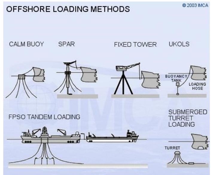
Fig. 1 Sketch of different offshore loading/unloading methods. (IMCA, 2003)
