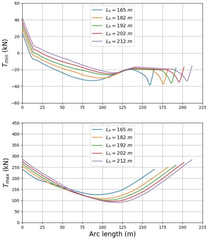
Fig. 17 Dynamic tension envelope curves (minimum and maximum) along the loading hose arc length,  $L_h$  varies from 165 m to 212 m.  $D_h = 100$  m. FSO at the left side, CNG vessel at the right side.
