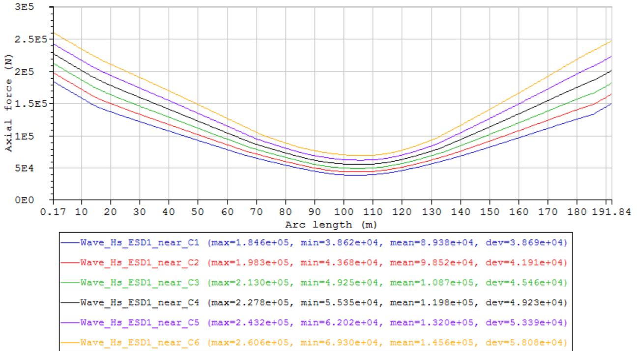
Figure 29 Maximum axial force envelope curves of the cases in Condition set – Wave\_Hs\_ESD1\_near (Table 15).
