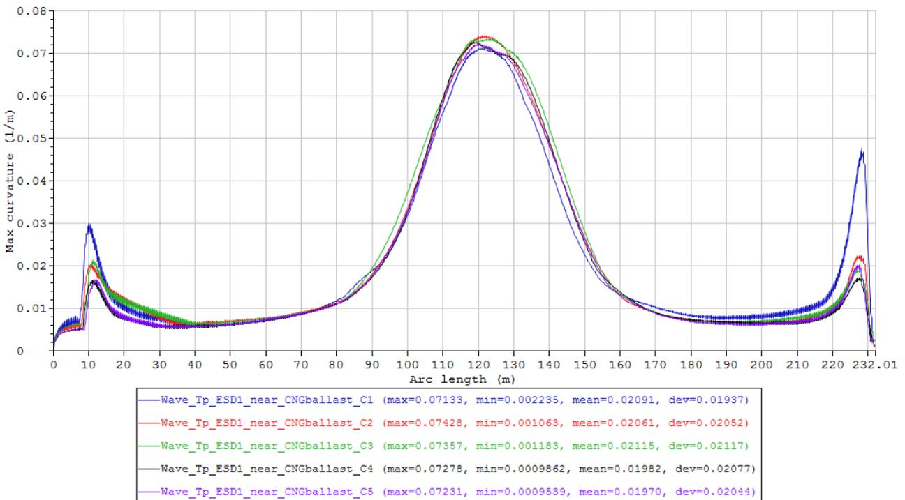
Figure 82 Maximum curvature envelope curves of the cases in Condition set – Wave\_Tp\_ESD1\_near\_CNGballast (Table 23).
