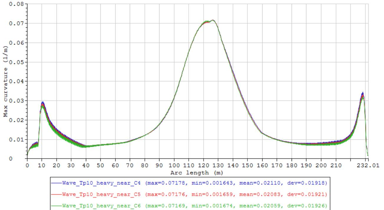
Figure 64 Maximum curvature envelope curves of the cases in Condition set – Wave\_Tp10\_heavy5\_near, last 3 cases with mass/length variation (Table 19).
