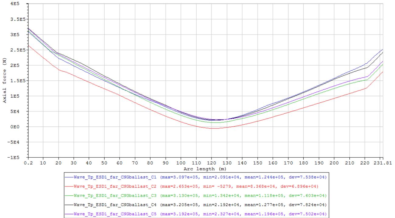
Figure 87 Minimum axial force envelope curves of the cases in Condition set – Wave\_Tp\_ESD1\_far\_CNGballast (Table 23).
