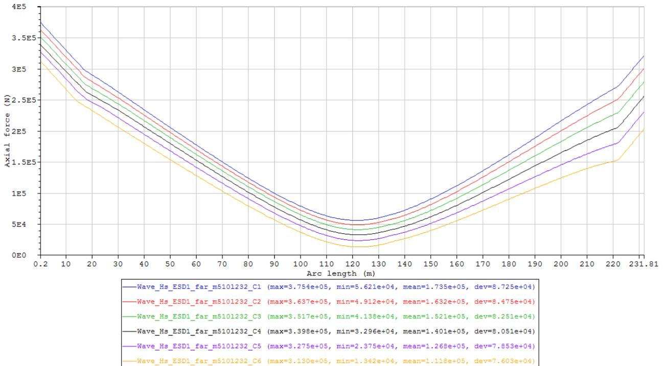
Figure 72 Minimum axial force envelope curves of the cases in Condition set – Wave\_Hs\_ESD1\_far\_m5101232 (Table 21).
