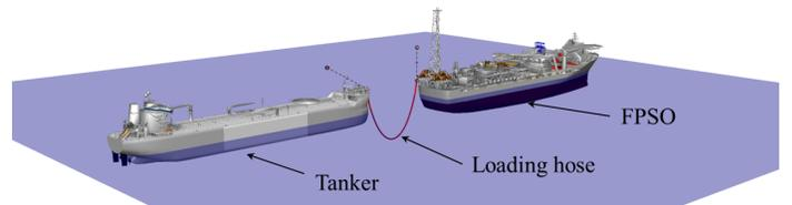
Fig. 2 A typical tandem offshore loading system. (Yin et al., 2017)
