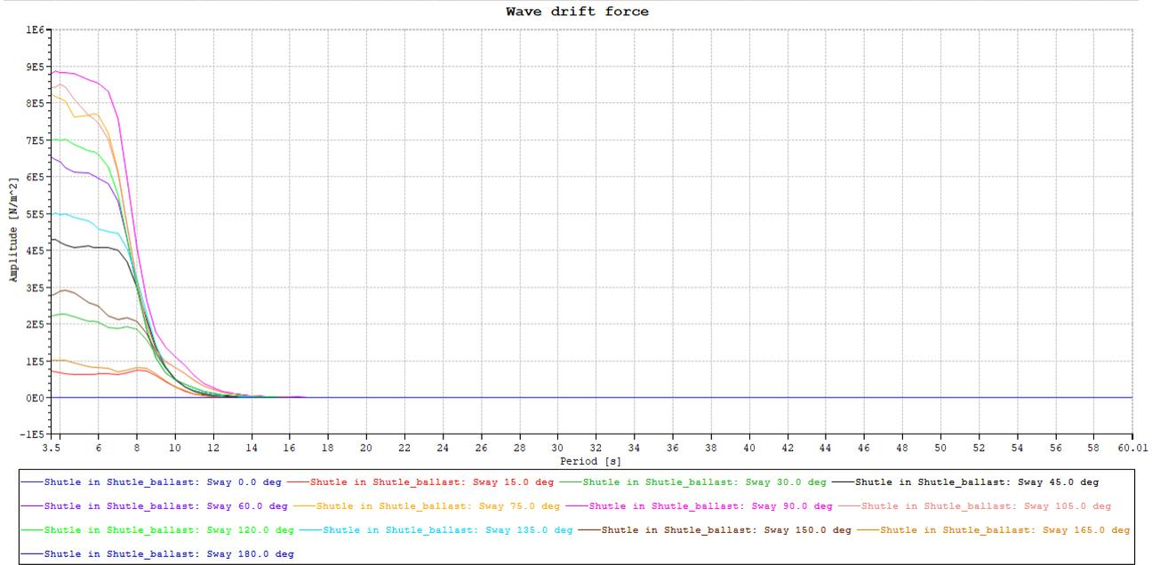
Figure 98 Sway wave drift force for GASVESSEL.
