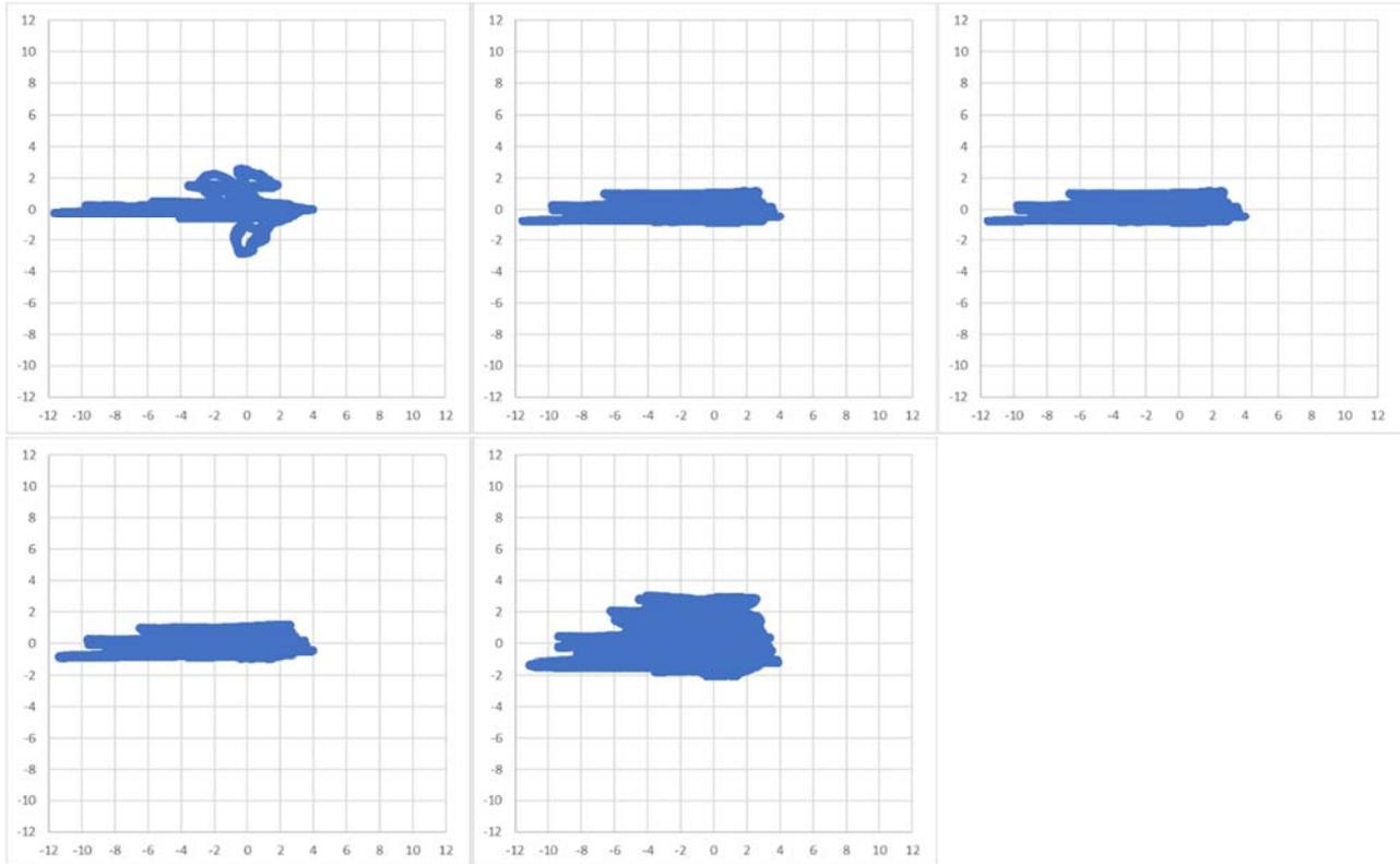
Figure 18 Surge (vertical) and sway (horizontal) motion relative to mean GASVESSEL position, for all  $T_p$  for the five environment cases in Table 29.
