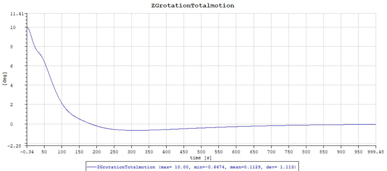
Figure 13 The step response for the heading with SIMO internal DP with gain corresponding to a natural period of 145 sec.
