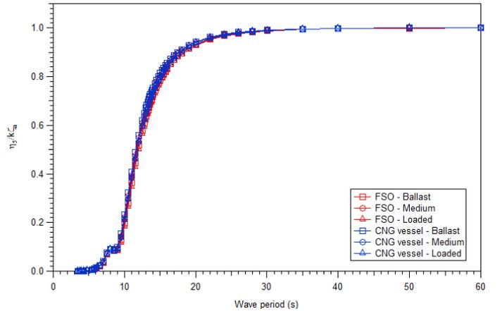
Fig. 8 Pitch motion RAOs for the different hull variants and loading conditions in head waves ( $\beta = 180$  deg). The pitch RAO is given in rad/m.
