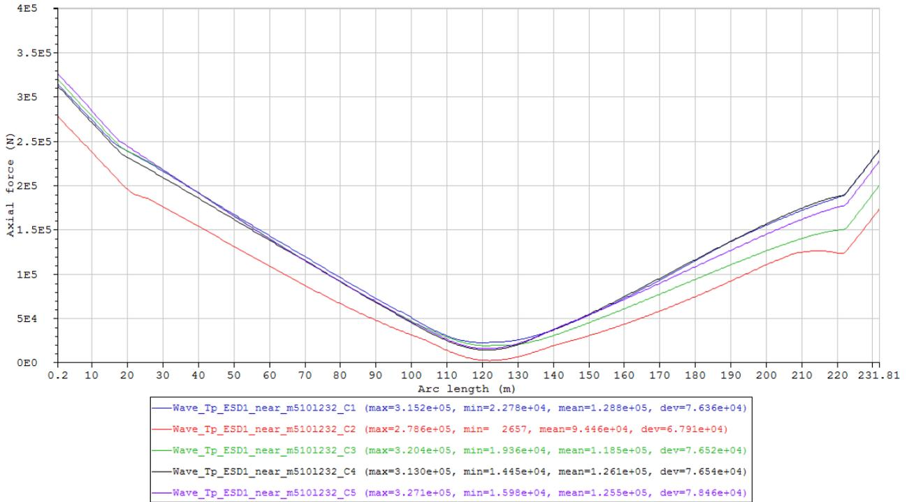
Figure 75 Minimum axial force envelope curves of the cases in Condition set – Wave\_Tp\_ESD1\_near\_m5101232 (Table 21).
