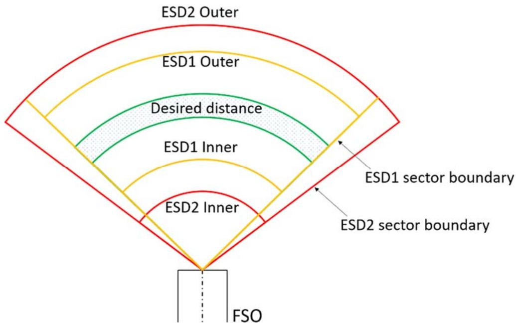
Figure 14 Illustration of offloading sectors behind FSO.
