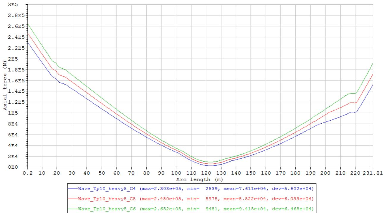
Figure 60 Minimum axial force envelope curves of the cases in Condition set - Wave\_Tp10\_heavy5, last 3 cases with mass/length variation (Table 19).
