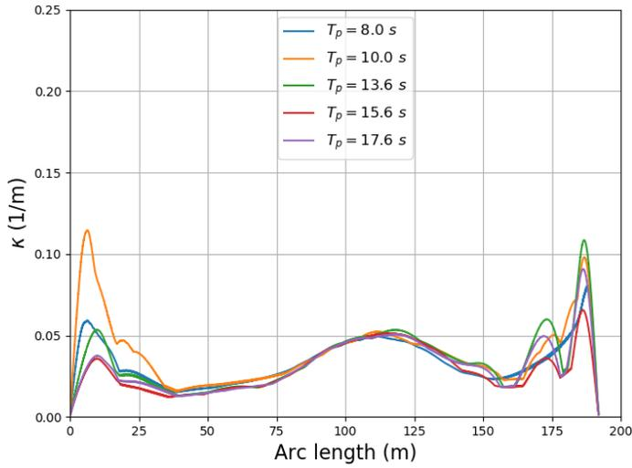
Fig. 20 Dynamic curvature envelope along the loading hose arc length.  $T_p$  varies from 8.0 s to 17.6 s,  $H_s = 6$  m.  $L_h = 192$  m,  $D_h = 100$  m. FSO at the left side, CNG vessel at the right side.
