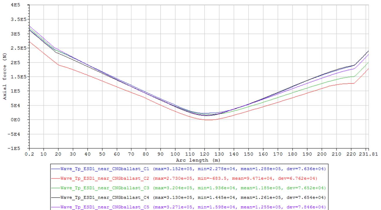
Figure 84 Minimum axial force envelope curves of the cases in Condition set – Wave\_Tp\_ESD1\_near\_CNGballast (Table 23).
