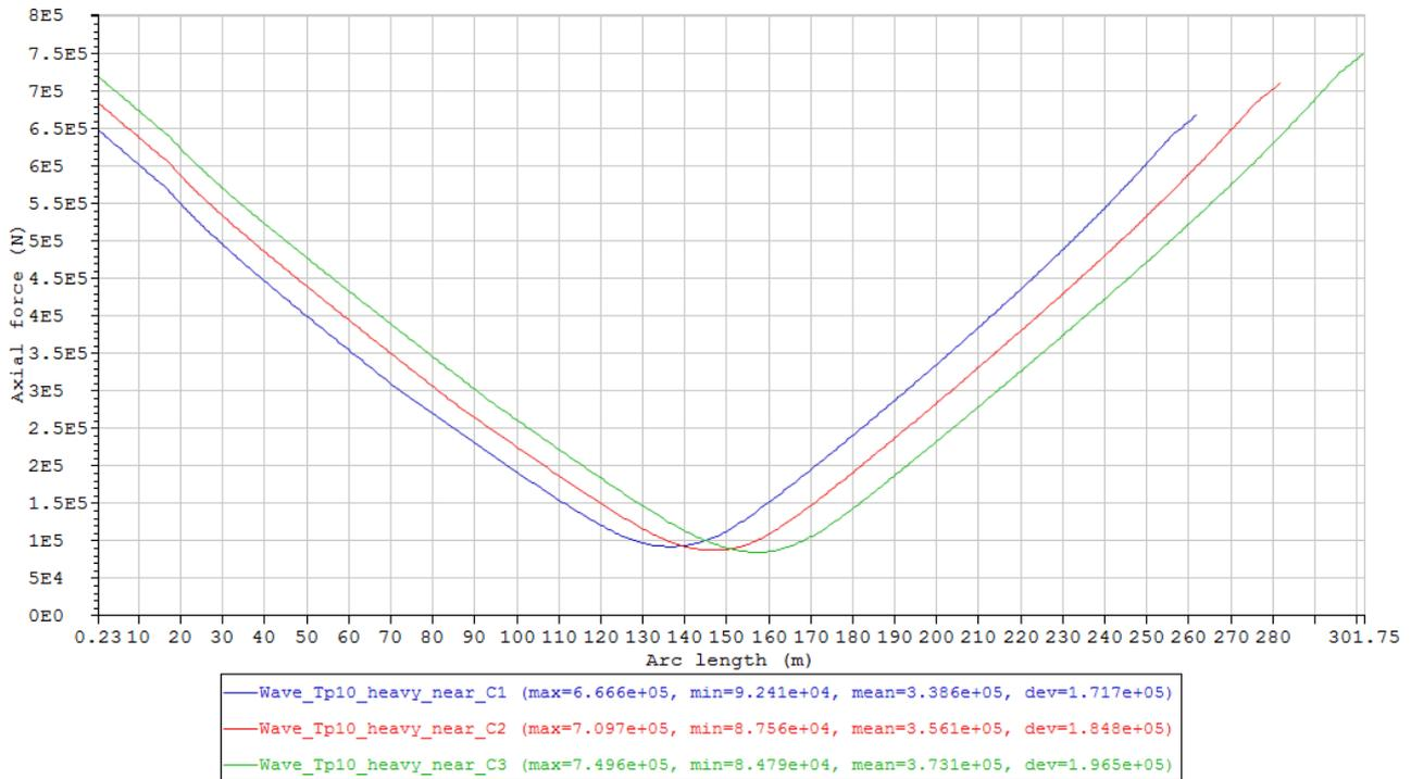
Figure 62 Maximum axial force envelope curves of the cases in Condition set - Wave\_Tp10\_heavy5\_near, first 3 cases with length variation (Table 19).
