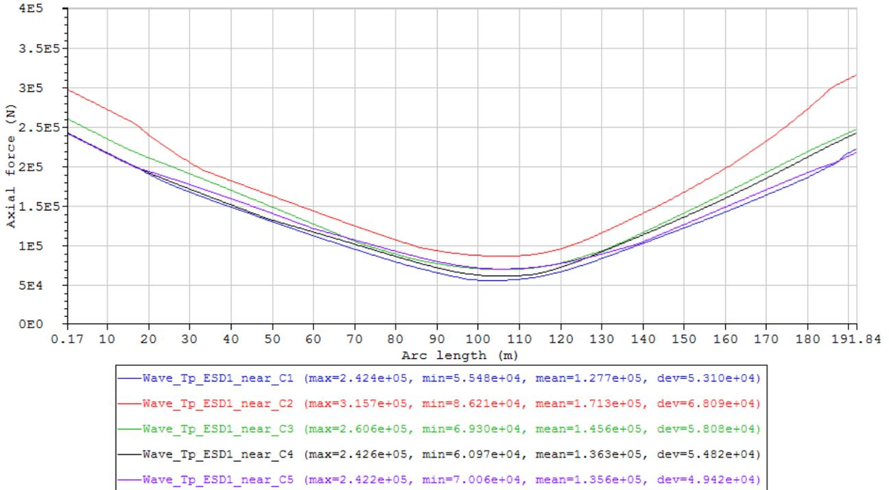
Figure 35 Maximum axial force envelope curves of the cases in Condition set – Wave\_Tp\_ESD1\_near (Table 15).
