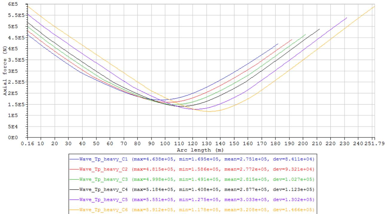
Figure 41 Maximum axial force envelope curves of the cases in Condition set – Wave\_Tp\_heavy (Table 17).
