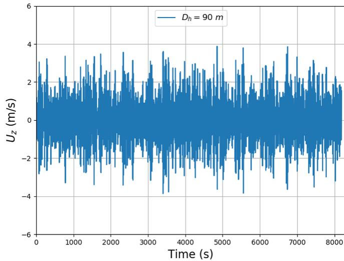
Fig. 15 Dynamic heave motion time series of CNG vessel bow,  $D_h = 90$  m,  $L_h = 115$  m.
