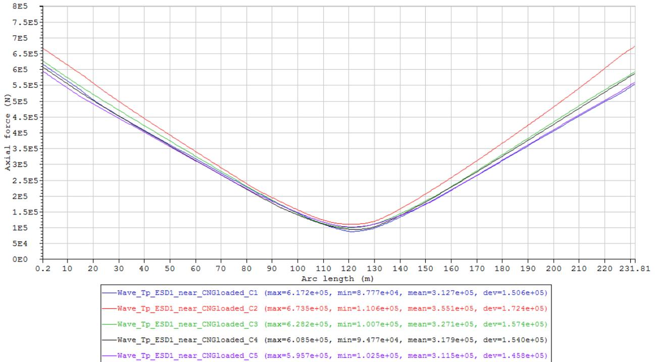
Figure 89 Maximum axial force envelope curves of the cases in Condition set – Wave\_Tp\_ESD1\_near\_CNGloaded (Table 23).
