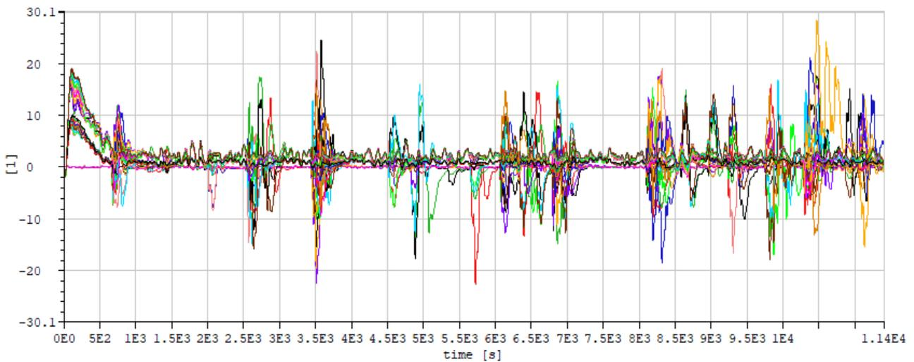
Figure 24 Hose angle behind FSO. The ESD sector is  $\pm 30$  deg.
