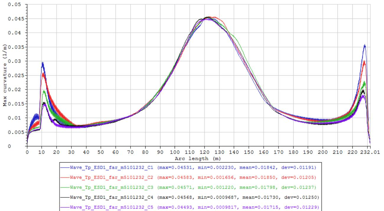
Figure 76 Maximum curvature envelope curves of the cases in Condition set – Wave\_Tp\_ESD1\_far\_m5101232 (Table 21).
