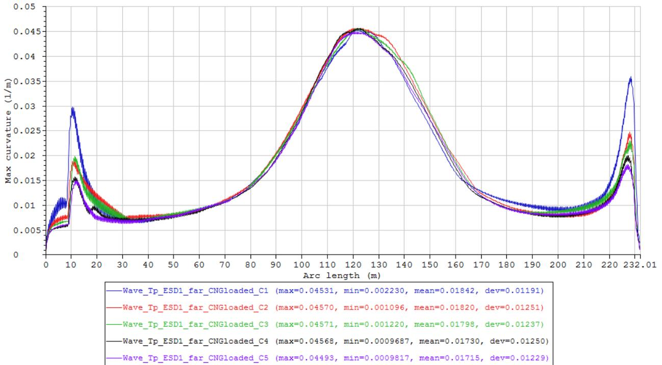
Figure 91 Maximum curvature envelope curves of the cases in Condition set – Wave\_Tp\_ESD1\_far\_CNGloaded (Table 23).
