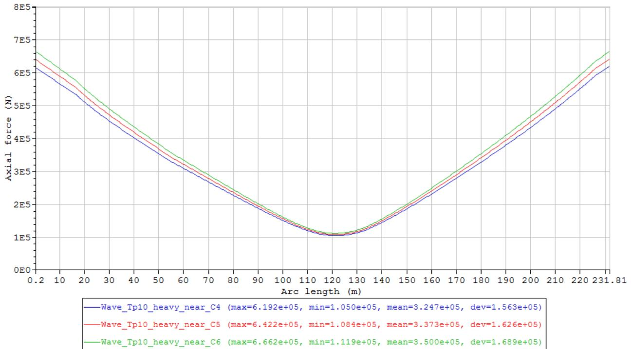
Figure 65 Maximum axial force envelope curves of the cases in Condition set – Wave\_Tp10\_heavy5\_near, last 3 cases with mass/length variation (Table 19).
