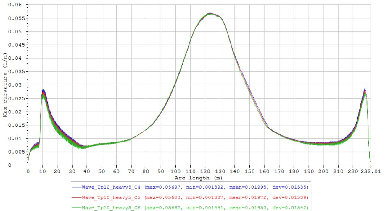
Figure 58 Maximum curvature envelope curves of the cases in Condition set – Wave\_Tp10\_heavy5, last 3 cases with mass/length variation (Table 19).
