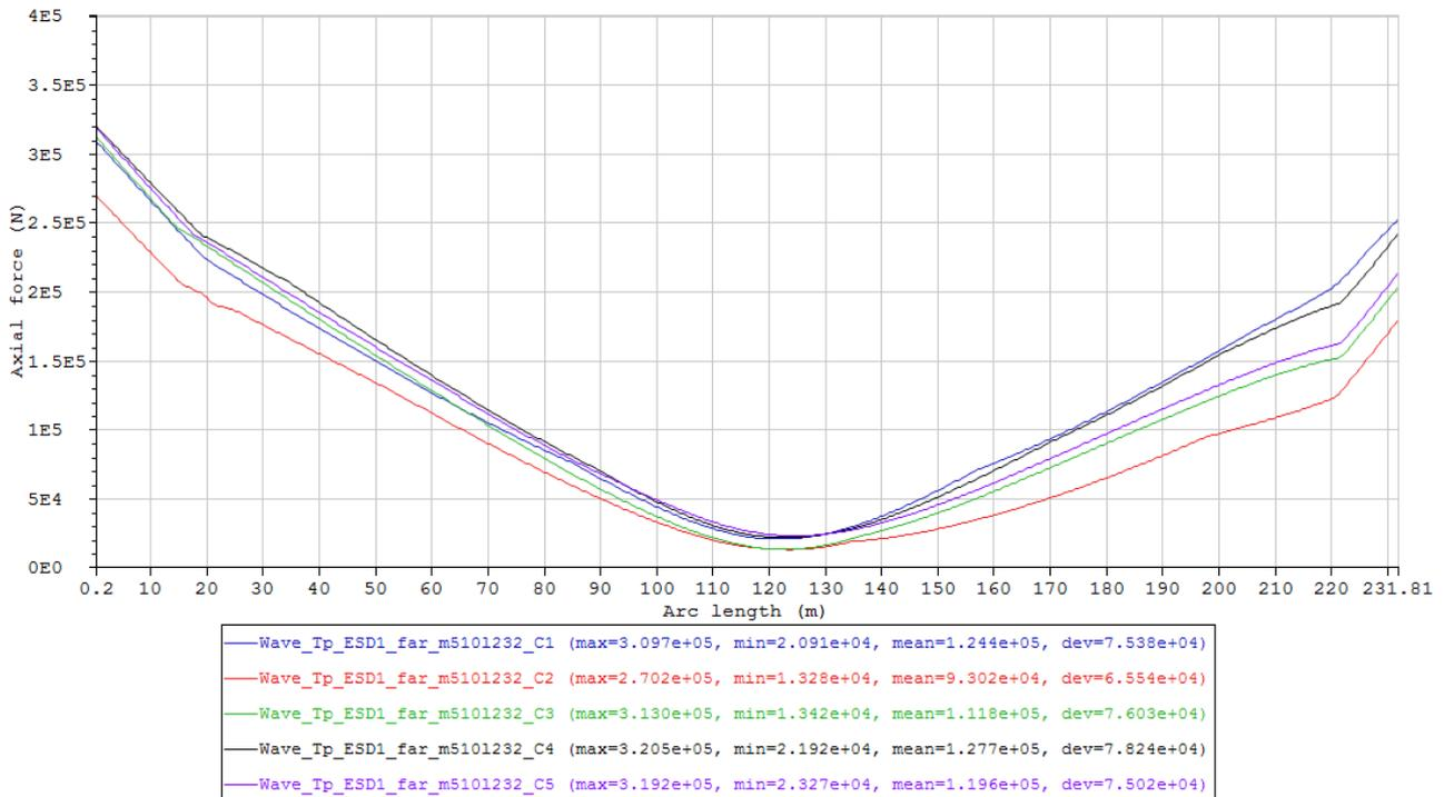
Figure 78 Minimum axial force envelope curves of the cases in Condition set – Wave\_Tp\_ESD1\_far\_m5101232 (Table 21).
