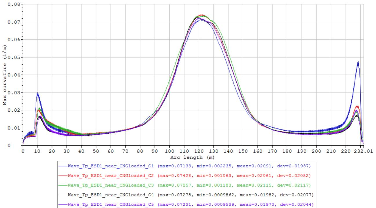
Figure 88 Maximum curvature envelope curves of the cases in Condition set – Wave\_Tp\_ESD1\_near\_CNGloaded (Table 23).
