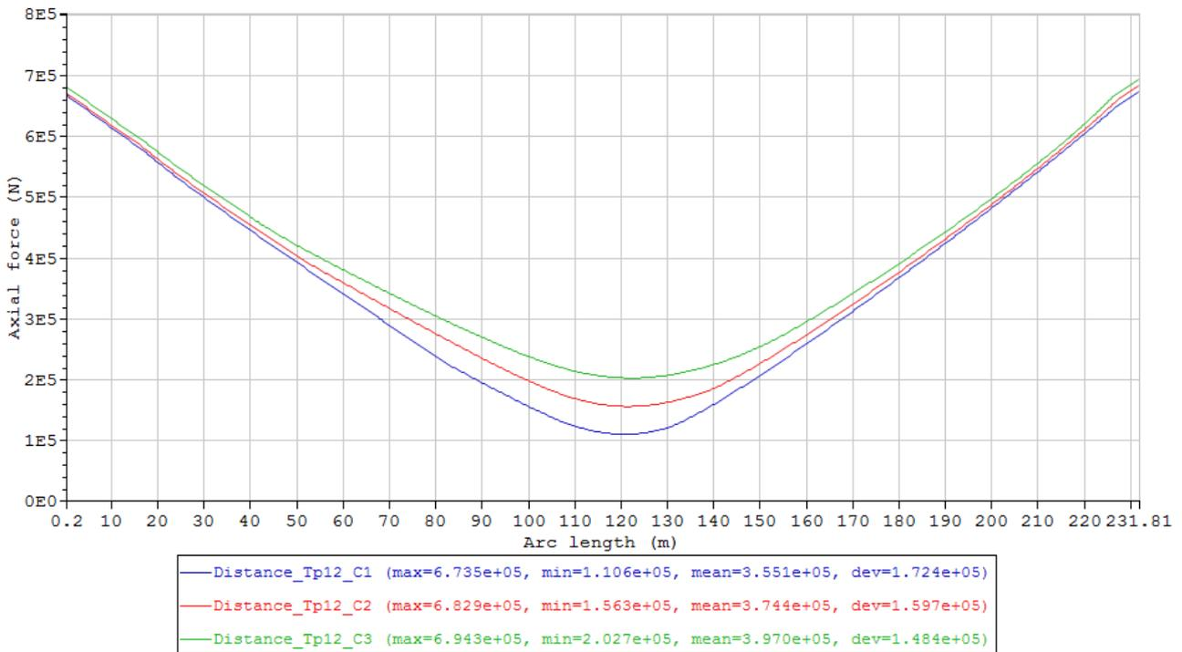
Figure 80 Maximum axial force envelope curves of the cases in Condition set – Distance\_Tp12 (Table 23).
