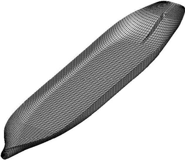
Fig. 6 Panel model for the CNG vessel with 5370 panels.
