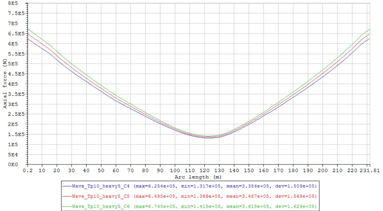
Figure 59 Maximum axial force envelope curves of the cases in Condition set - Wave\_Tp10\_heavy5, last 3 cases with mass/length variation (Table 19).
