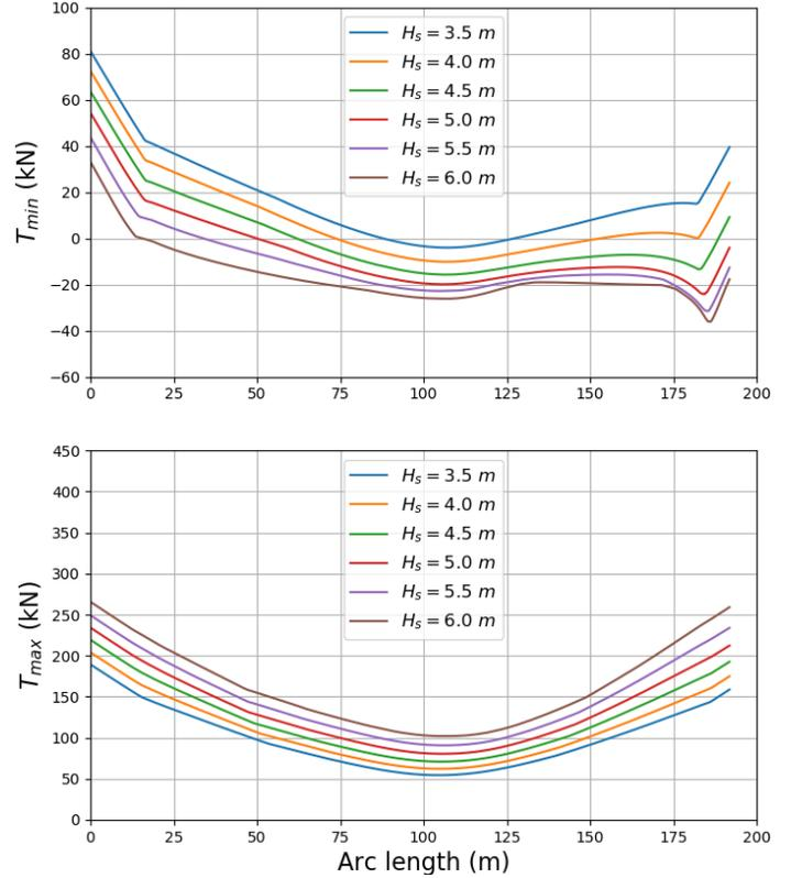
Fig. 19 Dynamic tension envelope curves (minimum and maximum) along the loading hose arc length.  $H_s$  varies from 3.5 m to 6.0 m.  $L_h = 192$  m,  $D_h = 100$  m. FSO at the left side, CNG vessel at the right side.
