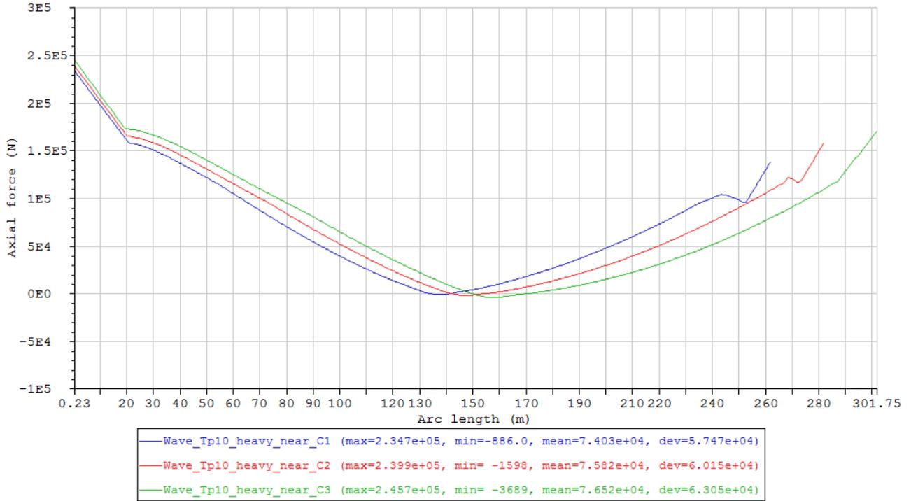
Figure 63 Minimum axial force envelope curves of the cases in Condition set - Wave\_Tp10\_heavy5\_near, first 3 cases with length variation (Table 19).
