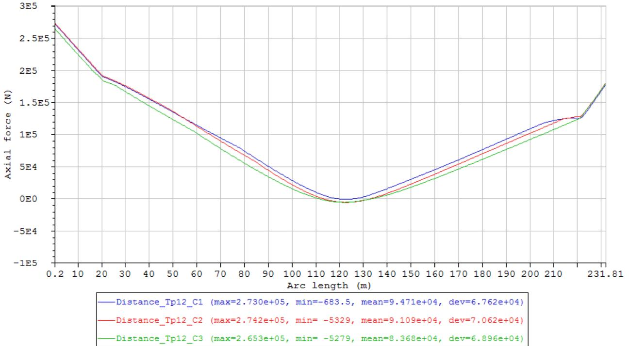
Figure 81 Minimum axial force envelope curves of the cases in Condition set – Distance\_Tp12 (Table 23).
