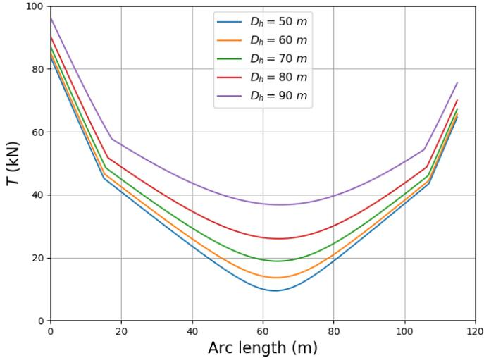
Fig. 12 Static tension along the loading hose arc length,  $D_h$  varies from 50 m to 90 m.  $L_h = 115$  m. FSO at the left side, CNG vessel at the right side.
