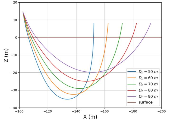
Fig. 10 Loading hose static profile,  $D_h$  varies from 50 m to 90 m.  $L_h = 115$  m. FSO at the left side, CNG vessel at the right side.
