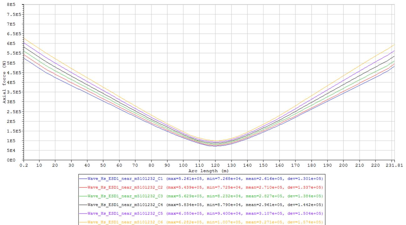
Figure 68 Maximum axial force envelope curves of the cases in Condition set – Wave\_Hs\_ESD1\_near\_m5101232 (Table 21).
