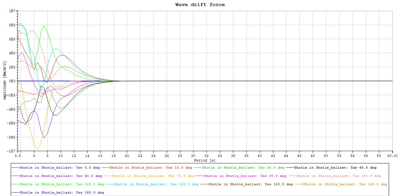
Figure 99 Yaw wave drift force for GASVESSEL.
