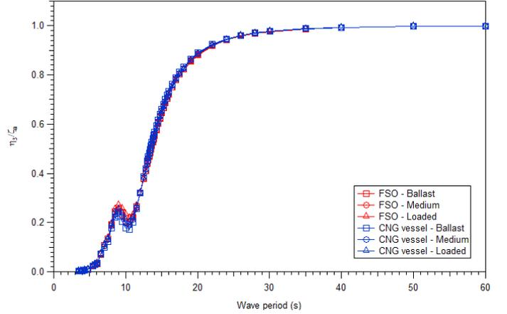
Fig. 7 Heave motion RAOs for the different hull variants and loading conditions in head waves ( $\beta = 180$  deg).
