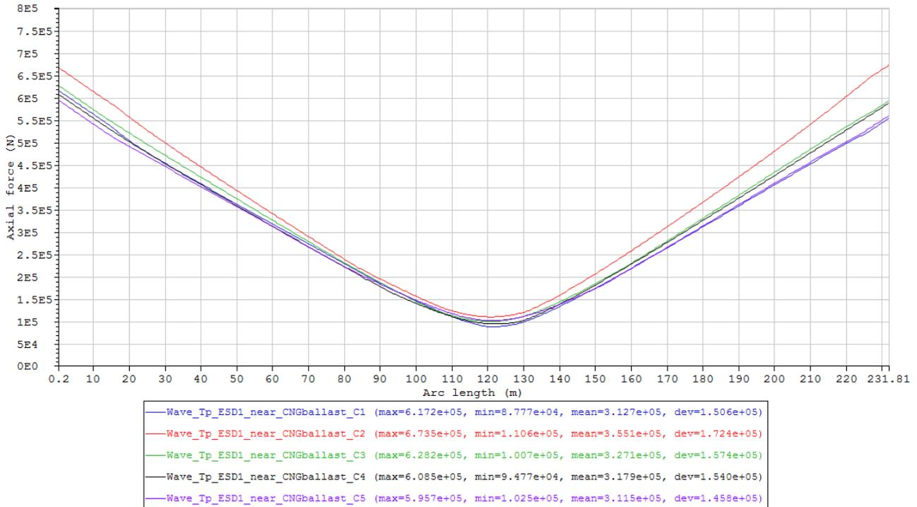
Figure 83 Maximum axial force envelope curves of the cases in Condition set – Wave\_Tp\_ESD1\_near\_CNGballast (Table 23).
