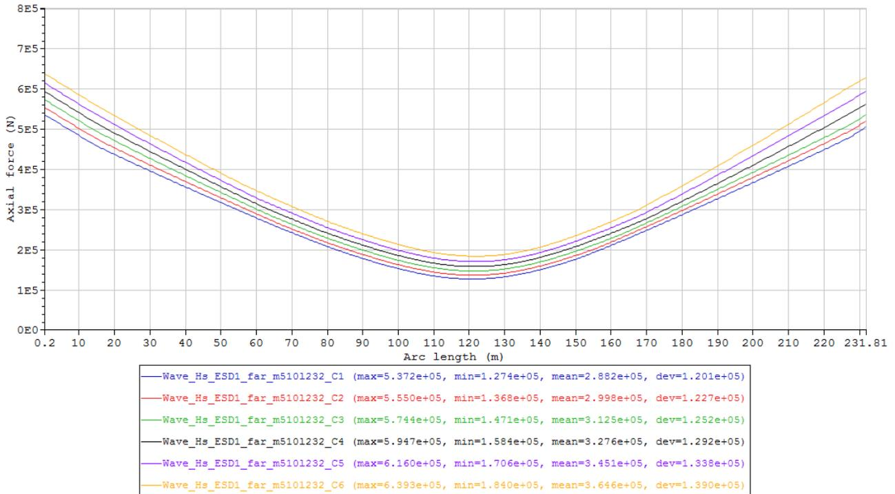
Figure 71 Maximum axial force envelope curves of the cases in Condition set – Wave\_Hs\_ESD1\_far\_m5101232 (Table 21).
