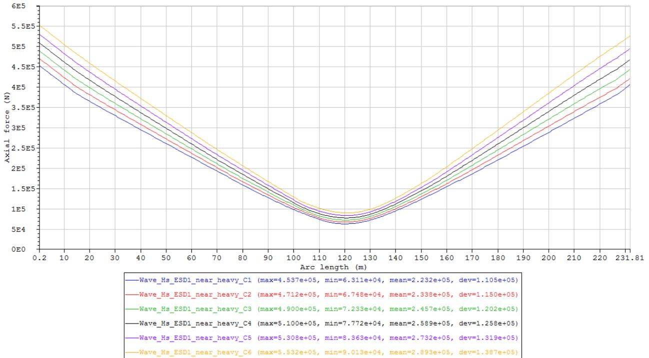
Figure 44 Maximum axial force envelope curves of the cases in Condition set – Wave\_Hs\_ESD1\_near\_heavy (Table 17).
