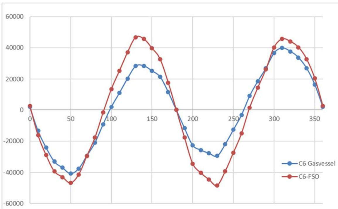
Figure 11 Wind coefficients [Ns<sup>2</sup>/m] for yaw-moment as function of SIMO heading for FSO and GASVESSEL. The GASVESSEL is less directionally unstable than the FSO for head wind (180 deg).
