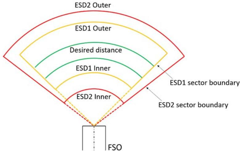
Figure 9 Illustration of offloading sectors behind FSO.
