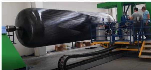
Figure 3. Prototype Gas Cylinders fabrication – Welding, Hydroforming, CF Winding
