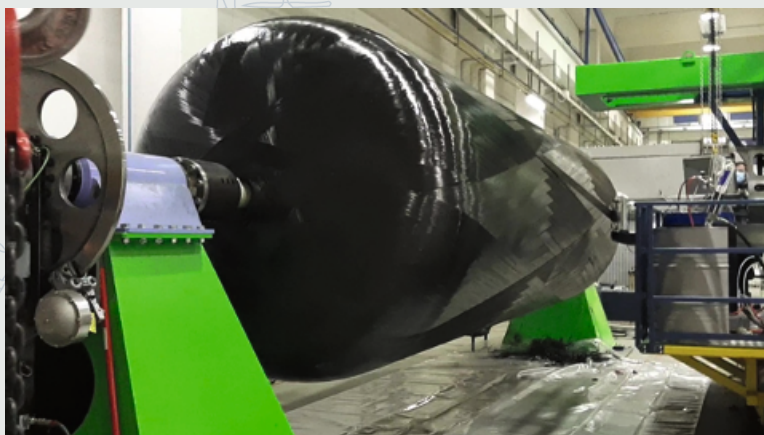
Figure 1. The cylinder is based on the Patent: WO2015 / 114549 A1 - Improved method to produce high-resistance composite vessels with inner metal liner and vessels made by said method. International Application No. PCT/IB2015/050668.
